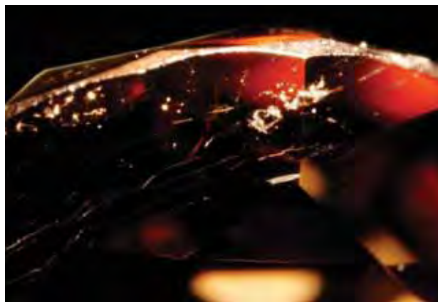
Figure 17. Thread-like and irregular fluid inclusions are visible through the bezel of this ferro-axinite. Photomicrograph by D. Beaton; field of view 7.2 mm.
