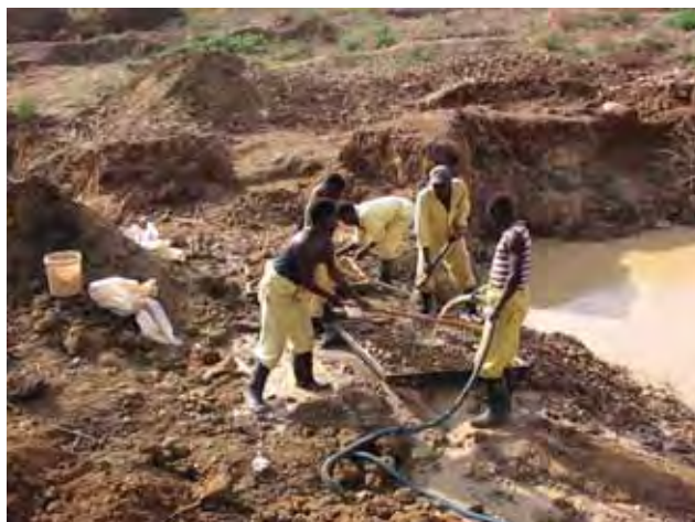
Figure 6. Secondary deposits downslope from the main Canary pegmatite are typically mined to a depth of 1–1.5 m (left). The miners recovered the gem rough by wet-screening the excavated material using water from a flooded mining pit (right). Photos by B. Anckar, June 2003.
