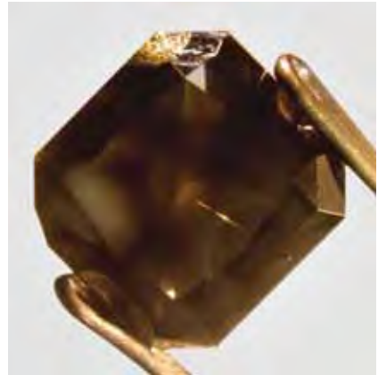
Figure 12. The 3.06 ct natural black diamond on the left, when viewed with strong transmitted light (right), shows an unusually long, straight etch channel as well as dark clouds of inclusions.
