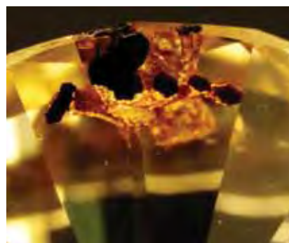
Figure 10. Multiple etch channels in the 0.57 ct diamond branch from the main channel, which breaks the surface of the table facet (0.55 × 0.6 mm; left). At this opening, it can be seen that the channel contains a transparent material that is completely surrounded by a dark brown material, which is responsible for the perceived color. Part of the main channel was also exposed on the crown facets, and cavities can be seen on its surface. The etch channels show roughly hexagonal outlines where they reach the pavilion surface (right).
