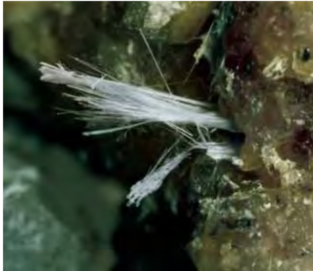
Figure 12. The fibrous crystals on this andradite specimen were identified as a mixture of calcite and asbestiform amphiboles. Photomicrograph by J. I. Koivula; field of view ~5.1 mm.
