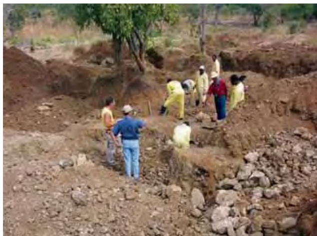
Figure 6. Secondary deposits downslope from the main Canary pegmatite are typically mined to a depth of 1–1.5 m (left). The miners recovered the gem rough by wet-screening the excavated material using water from a flooded mining pit (right). Photos by B. Anckar, June 2003.
