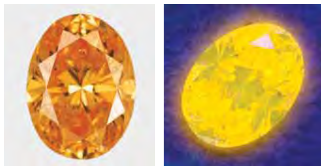
Figure 10. A 1.67 ct Fancy Vivid yellowish orange diamond, B56 (left), fluoresces moderate yellow-orange (center) with a long-wave UV lamp. The fluorescence spectra show a dominant peak at ~550 nm (i.e., category 3 fluorescence, right). The most intense fluorescence was recorded when excited by UV radiation at 325 nm. Photos by Jian Xin (Jae) Liao.
