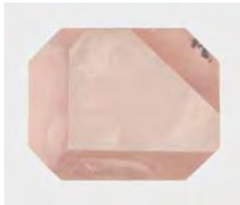
Figure 3. These two partially polished CVD crystals (1.05 and 1.20 ct) had a tabular morphology that is characteristic of CVD synthetic diamonds. Photos by Jian Xin (Jae) Liao.
