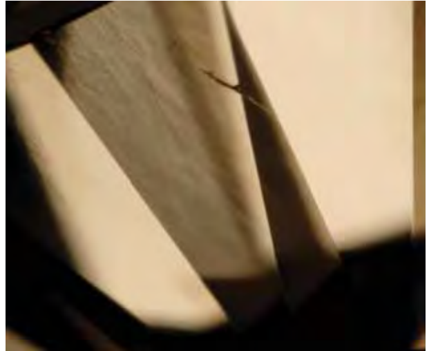
Figure 11. Internal graining was well developed but “fuzzy” in most of the CVD synthetic diamonds studied. Graining with clearly observable outlines, as seen here in sample AP-18, was rare. Photomicrograph by W. Wang; field of view 2.4 mm.
