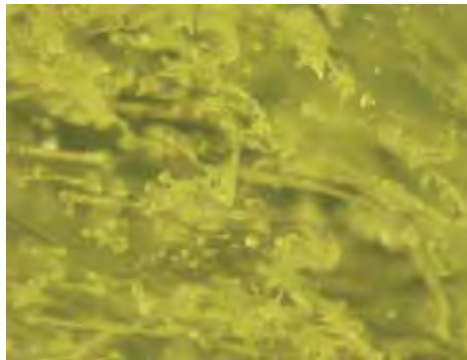
Figure 41. Numerous gas bubbles were present throughout the YAG, along with complex tube-like inclusions. Photomicrographs by C. Golecha; magnified 35× (left) and 30× (right).
