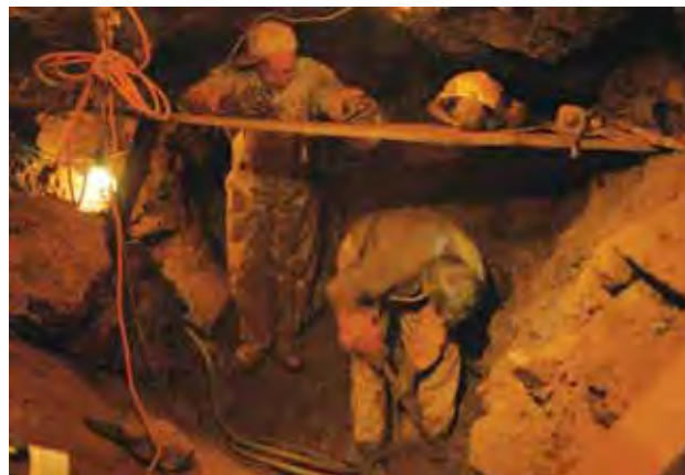
Figure 18. After several weeks of excavation, the cavity at Mt. Mica measured approximately 11 m long. A ramp was constructed for transporting buckets of pocket material through a small passageway into the main tunnel. Here, mine owner Gary Freeman digs material from the base of the pocket while miner Richard Edwards looks on. Note the mud-encrusted quartz crystals on the pocket wall in the right foreground. Photo by B. M. Laurs.
