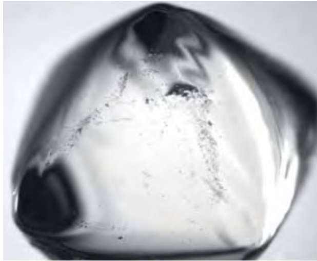
Figure 30. At first glance, this 1.53 ct rounded octahedron has the appearance of a rough diamond crystal. The granular surfaces seen along its edges raised suspicions about its origin, and it proved to have been manufactured from barium-rich glass. Photo by A. Respinger; magnified 16 \times .
