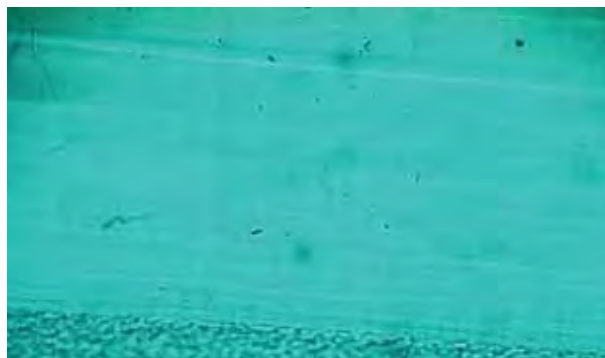
Figure 2. Straight, parallel growth bands, which also may be present in natural emeralds, are seen in this faceted Malossi synthetic emerald. Photomicrograph by Renata Marcon; magnified 30x.
