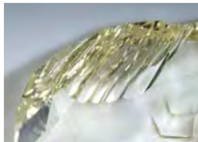
Figure 10. These facets, intended to represent the eagle's feathers, were cut by hand with a tool made expressly for this diamond. Magnified 8 \times .
