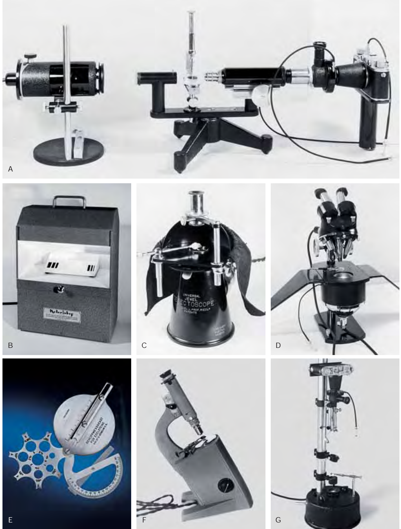
Figure 17. Dr. Gübelin developed a number of diagnostic gem-testing instruments during the 1940s and '50s, including: (A) the horizontal immersion photomicroscope, (B) the Koloriskop, (C) the Detectoscope, (D) the Gemmoscope, (E) the cut measuring device, (F) the Jewelers' Spectroscope, and (G) an innovative device that allowed the user to magnify and then photograph a gem's spectrum. With the exception of photo E, which was taken by Harold & Erica Van Pelt, all the other photos were commissioned or taken by Dr. Gübelin shortly after the development of the instrument.
