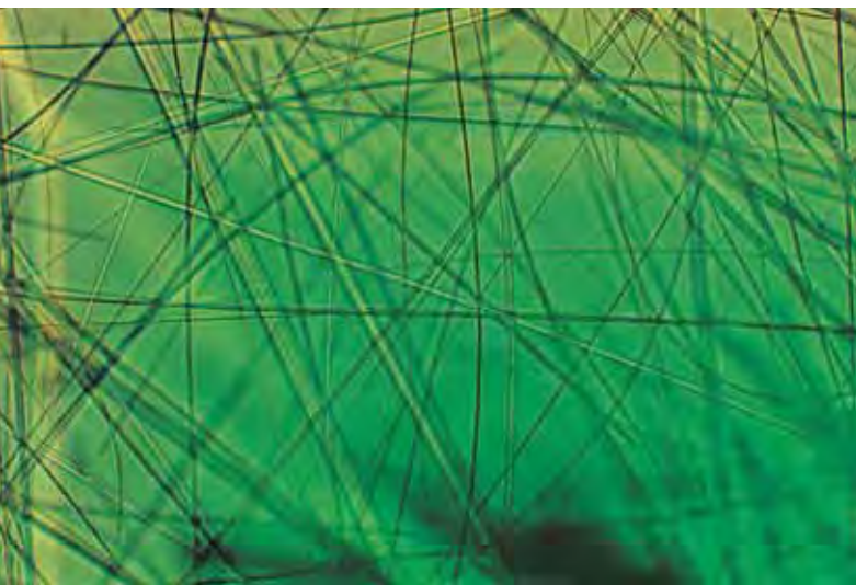
Figure 5. These amphibole fibers, which Dr. Gübelin believed were tremolite, are characteristic of emeralds from Sandawana, Zimbabwe. Photomicrograph by Edward J. Gübelin, magnified 20 \times , from the Photoatlas of Gemstone Inclusions (1986); used with permission from Opinio Verlag, Basel, Switzerland.
