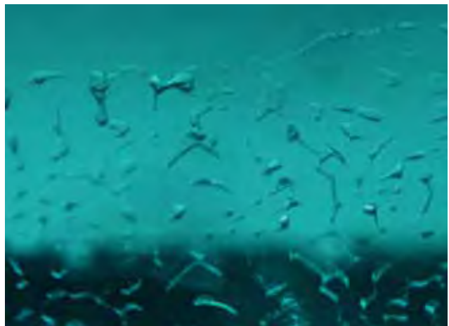
Figure 5. This faceted Malossi synthetic emerald contains conspicuous “fingerprints” (left) that are composed of tiny two-phase (liquid/gas) inclusions (right). Photomicrographs by Renata Marcon; magnified 8× (left) and 60× (right, in darkfield illumination).
