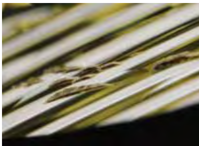
Figure 11. Many naturals were left along the girdle edge of the eagle's head to emphasize that the original rough had a shape similar to that of the finished stone. Magnified 38 \times .
