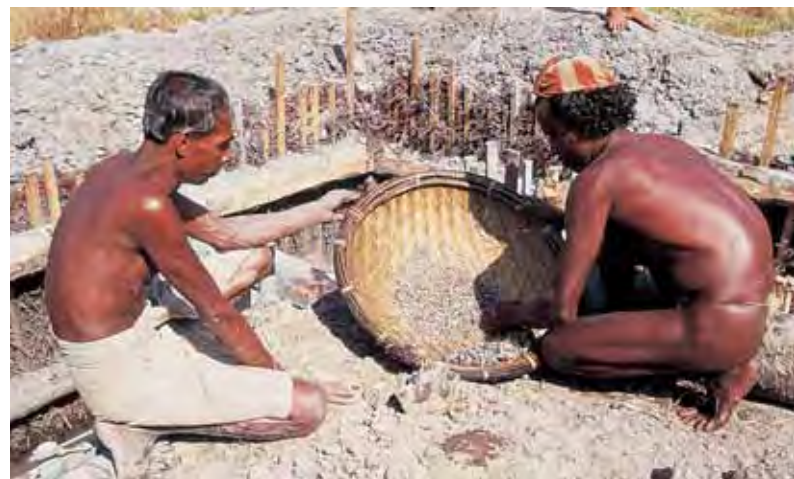
Figure 16. After washing of the illam (gem-bearing gravels), miners in Sri Lanka examine them for gem rough. Today, these time-honored recovery methods are still used by many gem miners in Sri Lanka and elsewhere. Photo by Edward J. Gübelin, from the early 1960s.
