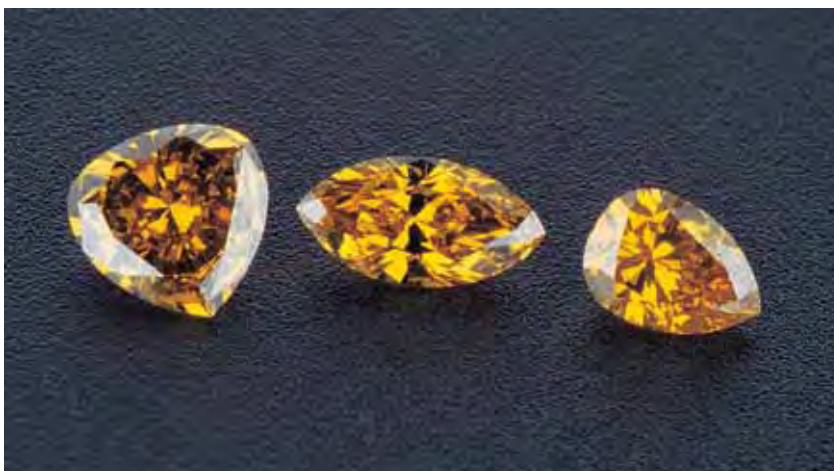
Figure 12. Due to their small size and lack of obvious synthetic characteristics, these three melee-size synthetic diamonds (0.11–0.16 ct) could be a challenge to identify outside a laboratory.
