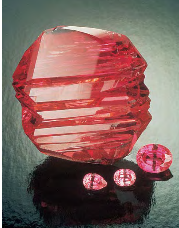
Figure 12. Chatham Created Gems produced this 884 ct flux-grown pink synthetic sapphire and the accompanying faceted material. Photo by Robert Weldon.
