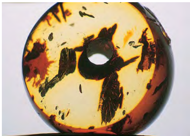
Figure 8. This heat-treated amber bead has been ground down on opposite sides to show that the color imparted by the treatment is confined to a thin surface layer. The dark brown hue fades on prolonged exposure to light. Photomicrograph by Shane F. McClure; magnified 10 \times .
