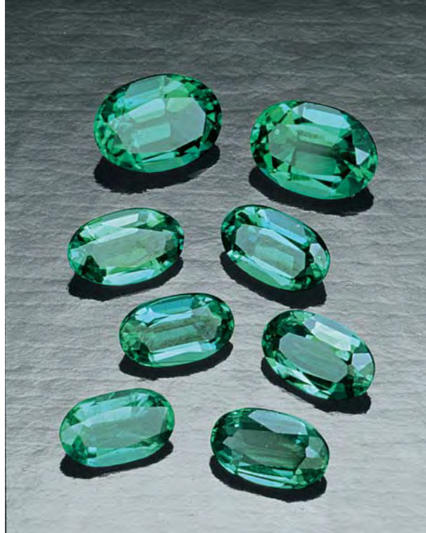
Figure 17. These hydrothermal synthetic emeralds (0.17–0.41 ct) were newly produced in Novosibirsk during the '90s, another product marketed by the Thai-Russian joint venture Tairus. Photo by Maha Tannous.
