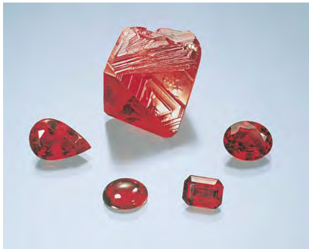
Figure 9. The properties of Douros flux-grown synthetic rubies (here the crystal is 44.74 ct and the faceted samples, 2.14–4.93 ct) closely resemble those of Ramaura synthetic rubies. Photo by Robert Weldon.
