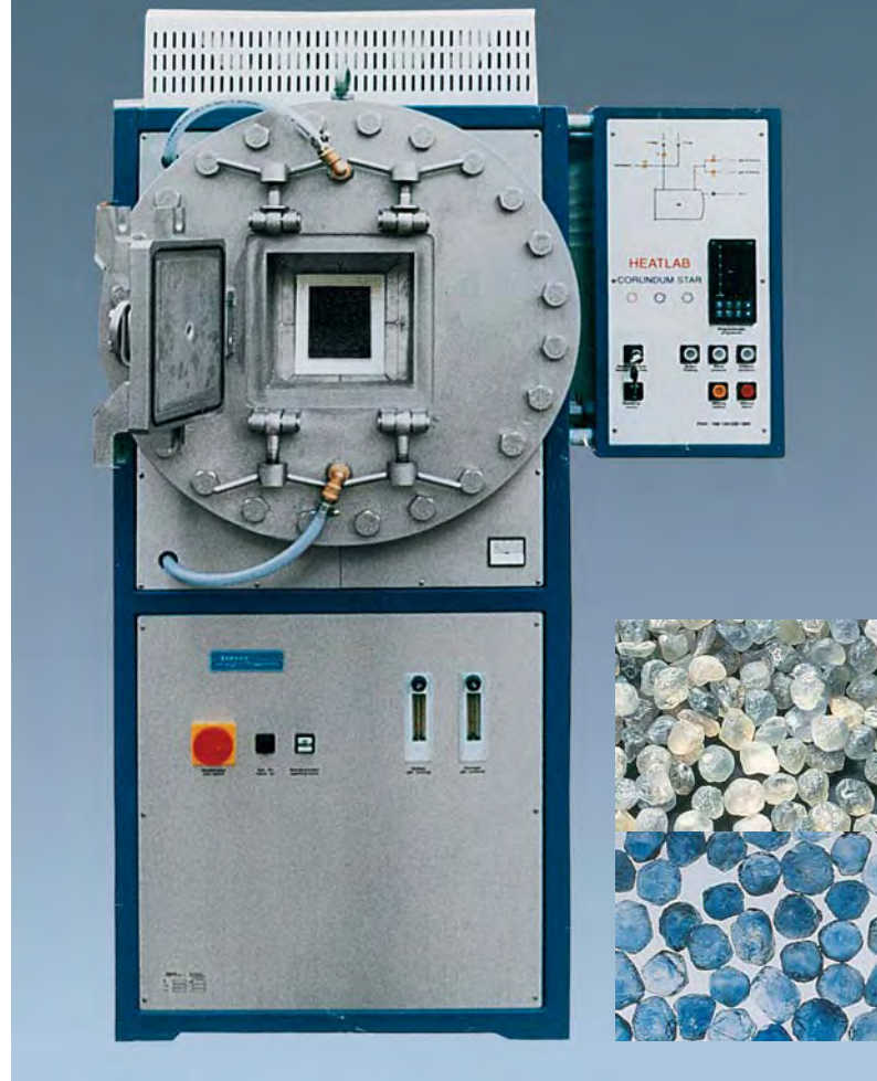
Figure 6. High-temperature furnaces such as this one were used with carefully controlled gas mixtures to perform heat treatment of rubies and yellow and blue sapphires (see inset for stones before [top] and after treatment; average size 4.5 mm). Furnace photo courtesy of Linn High Therm GmbH; inset photos © GIA and Tino Hammid (top) and © John L. Emmett (bottom).
