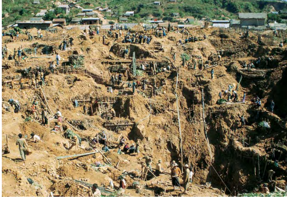
Figure 6. In Myanmar, rubies are mined from both primary and secondary (alluvial) deposits. At these alluvial workings near Mogok, a series of claims are explored by small groups of independent miners. Photo by Edward Boehm, March 1993.
