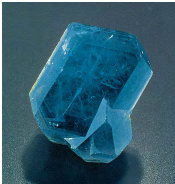
Figure 26. Irradiation is responsible for the blue color in this 20.38 ct crystal of synthetic sodalite from China. Photo by Robert Weldon.
