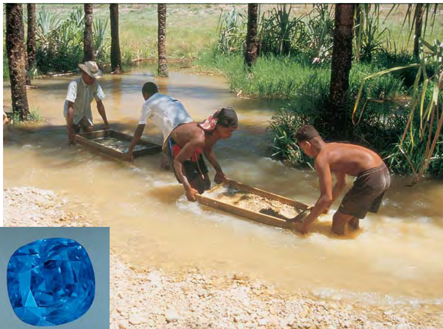
Figure 9. One of the most important gem discoveries of the decade occurred in south-central Madagascar at Ilakaka. Like Tunduru, these extensive alluvial deposits yielded several varieties of colored gems. Here, miners wet-sieve sediments in the Ilakaka River before removing gem minerals by hand; photo by Brendan M. Laurs, December 1999. Fine sapphires, such as the one that produced the 7.32 ct untreated Malagasy stone shown in the inset, are sometimes recovered. Sapphire courtesy of JOEB Enterprises and Pala International; photo © Harold & Erica Van Pelt.
