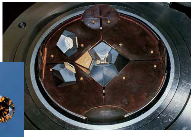
Figure 5. This BARS apparatus in Novosibirsk is typical of the split-sphere presses commonly used to manufacture Russian synthetic diamonds, such as the 0.04–1.07 ct samples in the inset. Shown here is the sample chamber as viewed from directly above. Photo of press by James E. Shigley; examples in inset courtesy of Alex Grizenko, photo by Maha Tannous.
