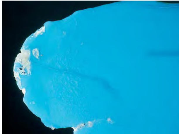
Figure 24. Although Zachery treatment can be proved only through chemical analysis, the presence of color concentrations along fractures in the turquoise is a good indication. Photomicrograph by Shane F. McClure; magnified 10 \times .
