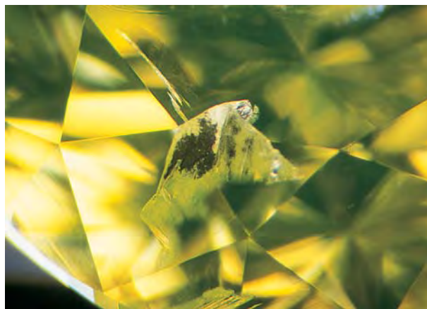
Figure 6. This fracture in an HPHT-annealed yellow-green diamond has partially graphitized, which is an indication that the stone has been subjected to high pressure/high temperature conditions. However, the presence of graphitization should not be construed as proof of treatment. Photomicrograph by Shane F. McClure; magnified 31 \times .
