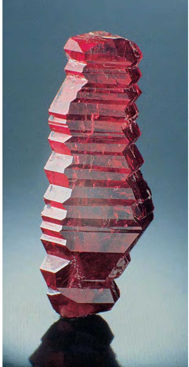
Figure 8. Knischka synthetic ruby crystals were grown in relatively large sizes, as evidenced by this 40.65 ct sample. Photo by Robert Weldon.
