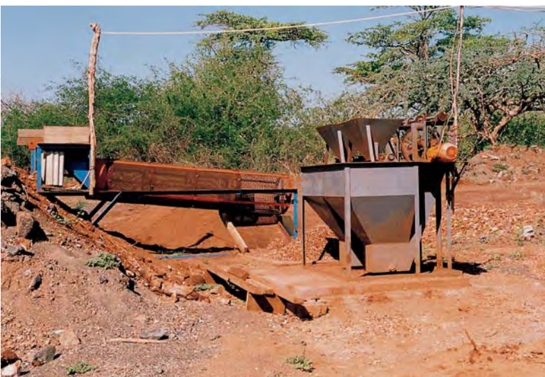
Figure 11. Simple crushing and sieving equipment was used to recover sapphires at the Sumai claims by Down to Earth Co. Photo by A. V. Seifert.
