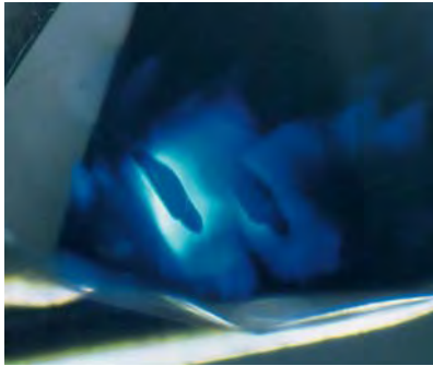
Figure 9. Magnification and fiber-optic lighting revealed both a dark blue color and a rod-shaped inclusion (typical of a metallic flux) in the synthetic diamond. Magnified 40 \times .
