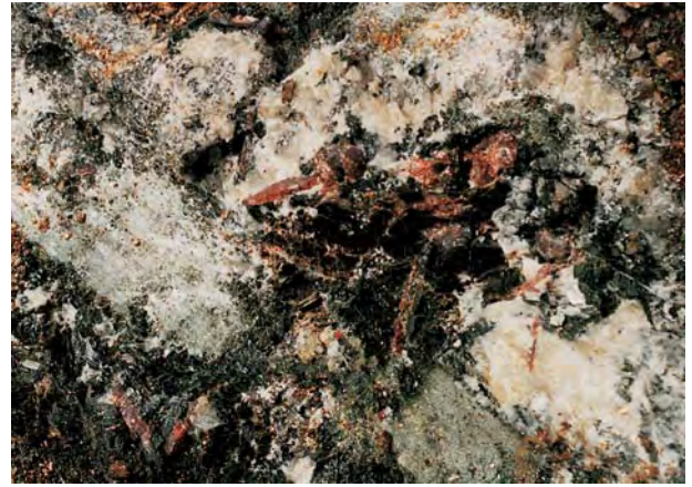
Figure 5. At the Cham-Shama claim, reddish orange sapphire crystals were recovered from desilicated pegmatites composed mainly of vermiculite (brown flakes), calcic plagioclase (white), and amphibole and chlorite (dark green). The prismatic sapphire crystal in the center of the photo is about 4 cm long. Photo by Varujan Arslanyan.
