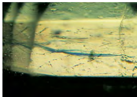
Figure 8. This 0.59 ct emerald filled with a mixture of epoxies (R.I. = 1.570) shows orange yellow (darkfield, left) and blue (brightfield, right) flash effects. Photomicrographs by John I. Koivula; magnified 15 \times .
