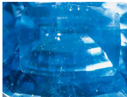
Figure 13. The 6.15 ct synthetic forsterite contained indistinct white inclusions that resemble dust particles, as well as pinpoints, tiny needles, and stringers. Magnified 11 \times .
