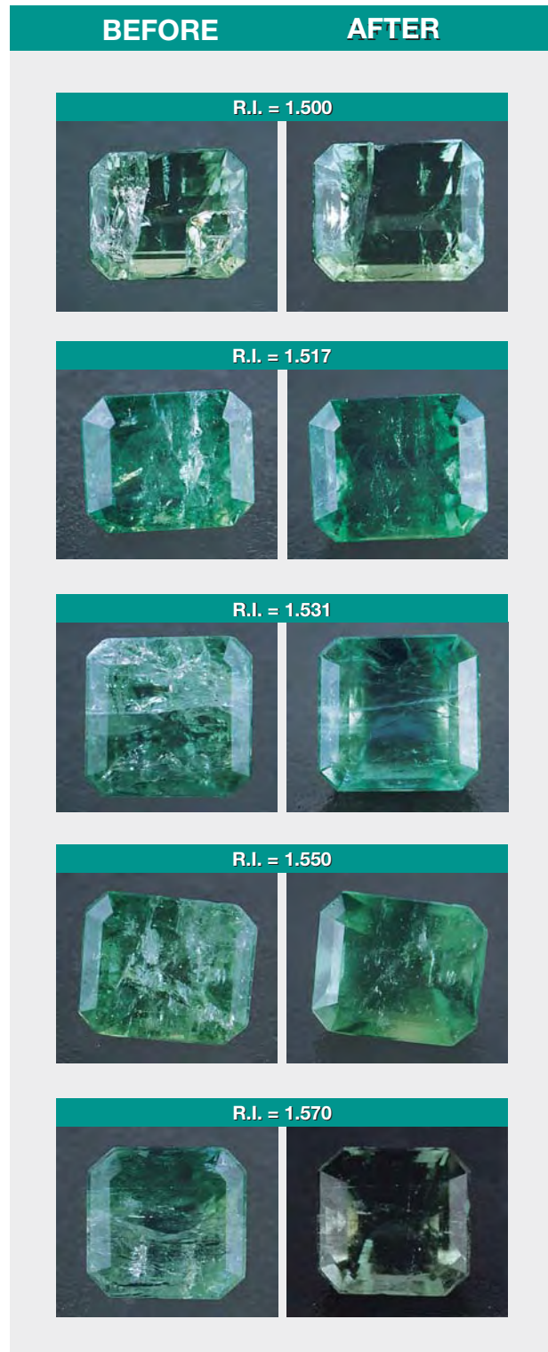
Figure 2. These before-and-after photographs illustrate that the fissures in emeralds become less visible as the R.I. of the filling material increases. Shown are fillers with R.I.'s of 1.500, 1.517, 1.531, 1.550, and 1.570. The refractive indices of the five emeralds ranged from 1.569 to 1.580. Photos by Maha DeMaggio.
