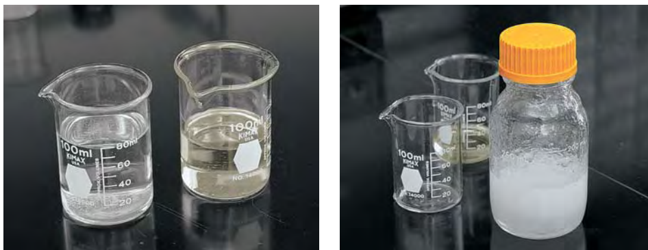
Figure 14. When water-insoluble filling substances (here, Araldite 6010) are mixed with water, they form a white cloudy emulsion. Left: Araldite 6010 and water before mixing; right: the substances shaken together. Photos by Maha DeMaggio.
