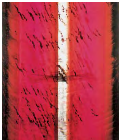
Figure 17. This 9.3-mm-wide crystal of hydrothermal synthetic beryl shows distinct color zoning, with a dark purplish blue rim and a purplish pink central area (left); these are the colors normally seen when observing the crystal. The colorless layer in the middle is the seed plate; the dark horizontal cracks are due to strain. A 90° rotation of the analyzer (right) produces a dramatic shift in the pleochroic colors, resulting in a reddish orange rim and an orangy red center. Photomicrographs by John I. Koivula.
