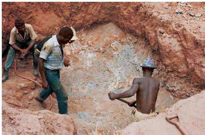
Figure 9. Miners work the desilicated pegmatite at the Cham-Shama claim from which reddish orange sapphire was recovered. The pegmatite is visible here as patches of white and greenish blue beneath the horizon of red lateritic soil. The hose to the left carried compressed air for removing the excavated material and cleaning the bottom of the pit. Photo by A. V. Seifert.
