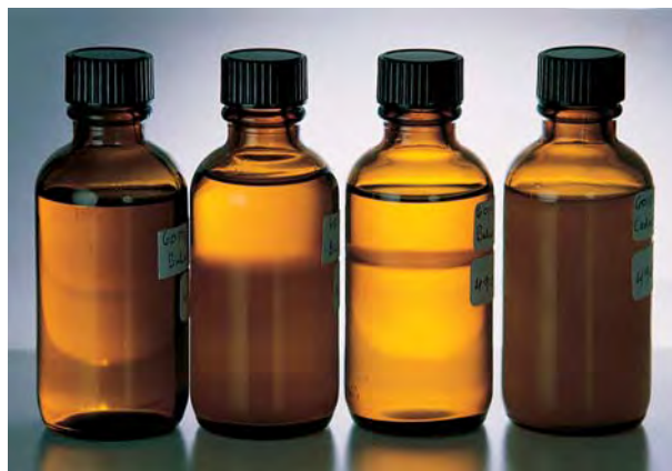
Figure 3. These four bottles of Baker cedarwood oil–Araldite 6010 mixtures show the unmixing of intermediate mixtures with 40% to 70% Araldite (left to right). Photo by Maha DeMaggio.
