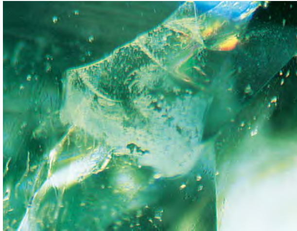
Figure 7. A white residue was seen deep within a fissure in this 0.47 ct emerald, which had been filled with a mixture of clove and cinnamon oils (R.I.= 1.570). Natural iridescence is also visible in this fissure (top of the image). Photomicrograph by John I. Koivula; magnified 20 \times .
