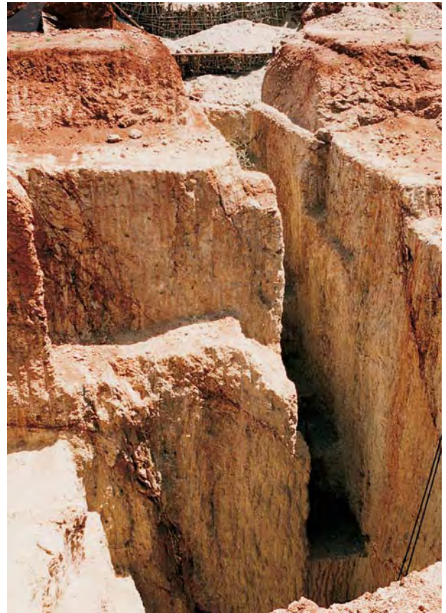
Figure 8. The deepest pit in the Kalalani area (40 m) was excavated for sapphire and ruby by Ruvu Gem Ltd., using a modified block mining method. Mining ceased here in 1994. Photo by A. V. Seifert.
