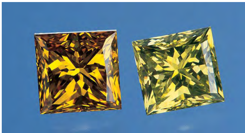
Figure 10. These two synthetic diamonds (0.59 and 0.63 ct) illustrate the range of color, from orangy yellow to greenish yellow, that was displayed by a group of 18 synthetic diamonds submitted to the laboratory at one time.
