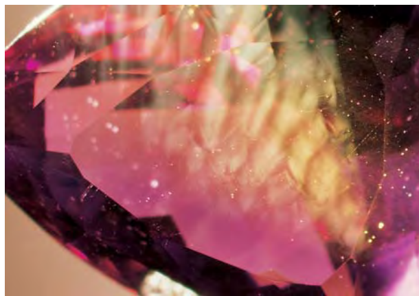
Figure 11. Stream-like structures are visible in the citrine portion of this 4.25 ct faceted synthetic ametrine. Photo by Taijin Lu.
