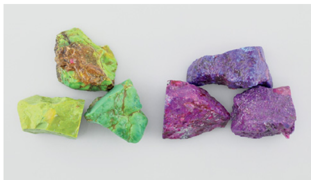
Figure 2. These rough samples of treated turquoise (5.75–10.11 g) show unusual colors and a polymer-like luster. Concentrations of colored polymer are visible as the yellow-brown area on the right corner of the upper yellow-green sample, and the red areas on the bottom purple to purple-pink samples. Photo by G. Choudhary.
