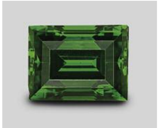
Figure 19. This 5.43 ct green sample proved to be calcium niobium gallium garnet, a lab-grown product with no natural counterpart. Photo by Bilal Mahmood.
