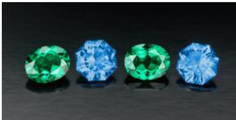
Figure 22. These four glass-ceramic samples (2.59–3.15 ct) were manufactured by Formica LLC. Photo by Robert Weldon.
