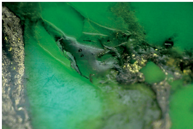
Figure 5. Polymer-filled areas and cavities in the turquoise appear to be indented and display a dull-to-waxy luster. Photomicrograph by G. Choudhary; magnified 45 \times .
