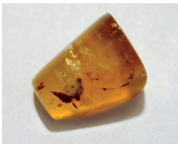
Figure 4. Opaque blebs, identified by SEM-EDS as hematite, are easily seen in this 11.03 ct opal, from which sample 19 was faceted. Photo by Andrea Pazzi.
