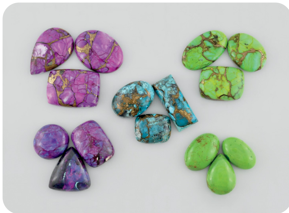
Figure 1. The 15 treated turquoise cabochons examined for this study are divided here into veined and unveined (or minimally veined) varieties that are purple to purple-pink (11.82–21.83 ct), yellow-green (8.10–18.12 ct), and blue (9.78–20.10 ct). Photo by G. Choudhary.
