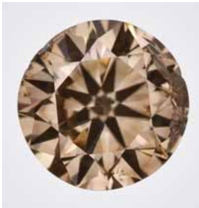
Figure 5. This 1.25 ct Fancy brown synthetic diamond proved to be CVD grown, but it had some unusual spectroscopic features.
