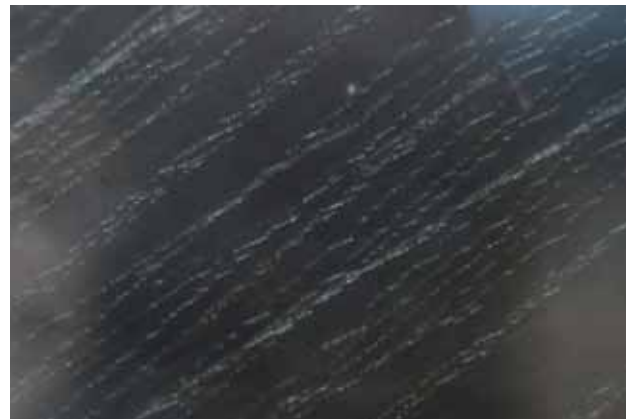
Figure 39. At relatively high magnification, linear trains of en echelon inclusions were visible in the sapphire. Photomicrograph by G. Choudhary; magnified 85 \times .
