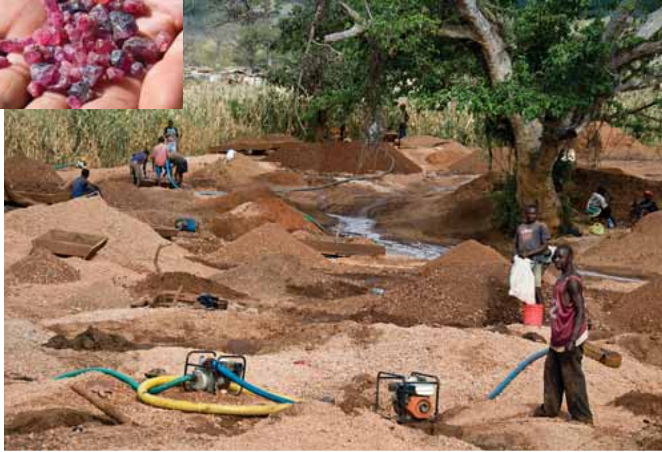
Figure 37. The eluvial soils are brought to the nearby river for washing, screening, and hand-picking of the ruby and sapphire. Photos by B. M. Laurs.
