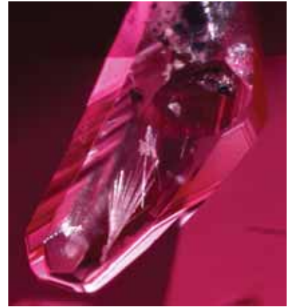
Figure 14. Another included crystal (identified as corundum) in the ruby contained a fan-shaped spray of needles. Field of view 0.63 mm.
