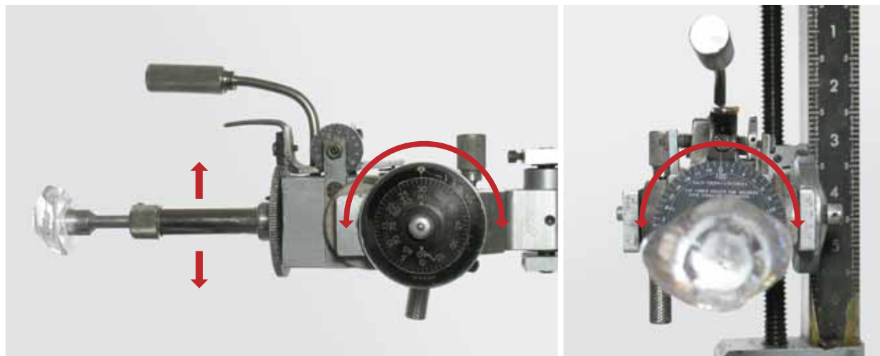
Figure 7. Each facet has a unique angle and index setting, as placement of the CZ model on this faceting machine illustrates. On the left: As the arm moves up and down, the angle dial rotates and displays the angle (0 reference is vertical). The arm position can be fixed at any angle setting to 0.25° accuracy. On the right: The arm is rotated about its longitudinal axis. Teeth on the gear behind the diamond allow any index setting to be fixed. A smaller wheel (the “index vernier” or “cheater,” shown above and to the left of the index dial in the image on the left) allows finer settings to less than 0.10° accuracy. Photos by S. Sucher.
