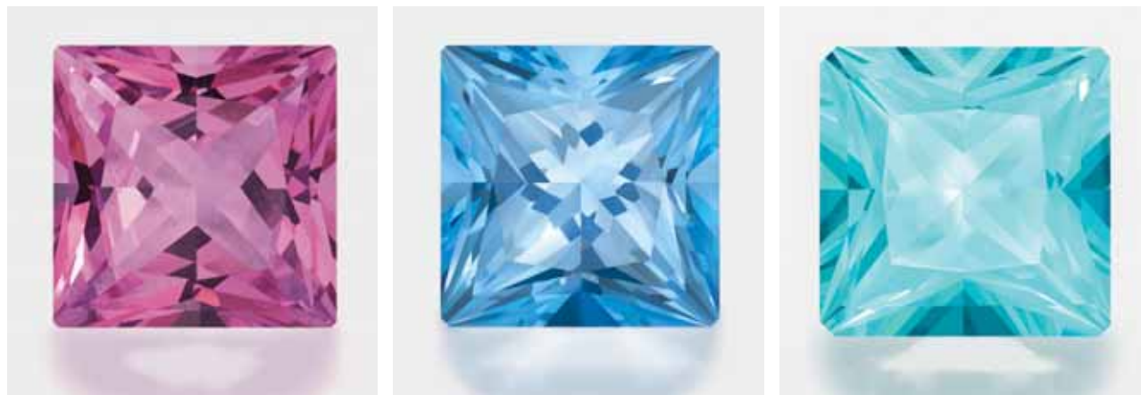
Figure 1. These three color-treated topazes were analyzed for this study: coated pink (left), diffusion-treated “Summer Blue” (middle), and diffusion-treated “Ice Blue” (right). All stones weigh 0.42 ct; photos by Tiroler Repro Druck.
