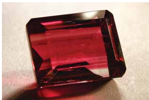
Figure 54. This 30.12 ct piece of faceted glass was sold as rubellite. The elongated straight lines are gas bubbles. Photo by B. Mocquet.
