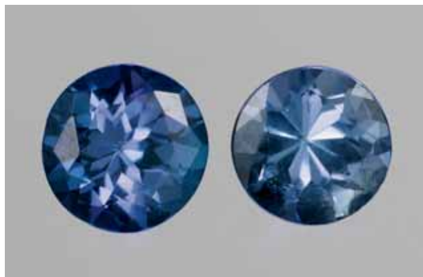
Figure 1. These two 5 mm stones were originally the same color. Repolishing of the one on the right resulted in a significant loss of color. Photo by C. D. Mengason.
