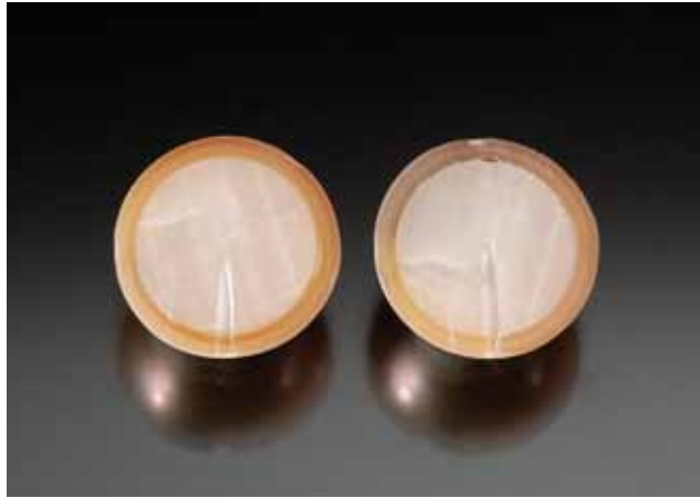
Figure 7. A 13.4 mm CBSB-nucleated round pearl sawn in half on the drill-hole axis revealed a 10.7 mm shell bead (left). An 11 × 23 mm CBSB-nucleated baroque pearl sawn in half on the long axis revealed a 9 mm shell bead (right). X-ray fluorescence and EDXRF tests proved the beads to be of saltwater origin. Courtesy of Sea Hunt Pearls; photos by Kevin Schumacher.
