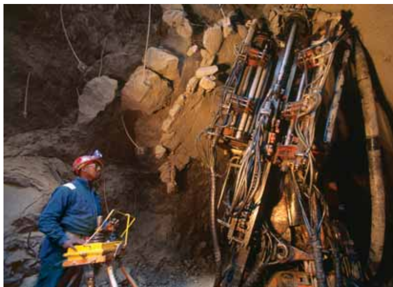
Figure 14. Open pit mines eventually reach a depth at which the costs of further recovery by open-pit mining exceed the revenue produced. The mine will either close or shift to underground mining if there are sufficiently valuable reserves to make it economic. This miner working underground in the De Beers Finsch mine is using an automatically synchronized operated multiple drill in preparation for planting explosives to blast out another mass of kimberlite. Photo © Hervé Collart/Sygma/Corbis.
