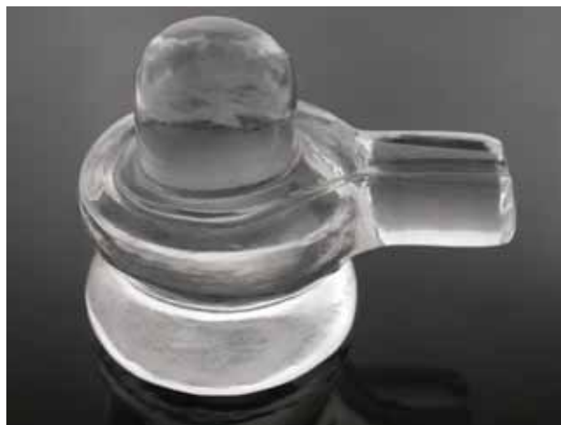
Figure 22. This 188 ct "Shivling," approximately 4.0 cm tall, was represented as rock crystal quartz, but proved to be manufactured glass. Photo by G. Choudhary.
