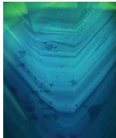
Figure 3. The nearly inert "trigons" in the blue fluorescing regions of this DiamondView image are rarely observed on polished facets of untreated natural diamonds.
