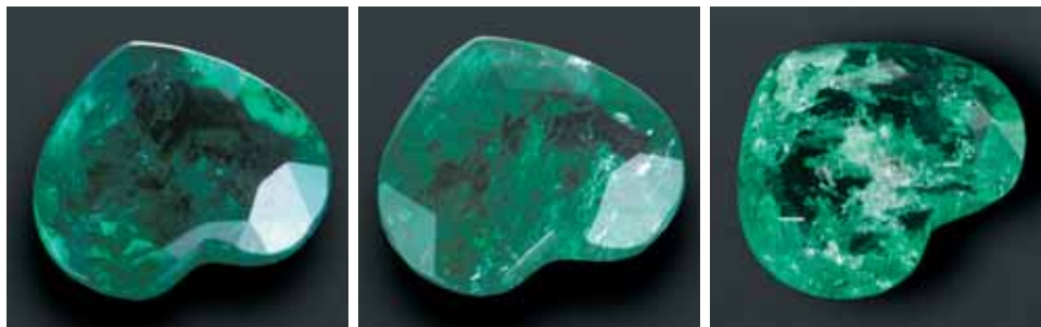
Figure 16. A 0.80 ct emerald filled with Araldite 6010 (no. 4797; left) showed obvious changes following a day in ethanol (center). After a day in acetone (right), not only did the fissures look empty, but there was also no evidence of filler in the emerald's FTIR spectrum.
