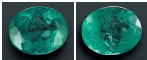
Figure 7. A 1.65 ct Gematrat-filled emerald (no. 4708; left, after filling) showed the most obvious change in the display-case test (right), with feathers opening up at the surface.
