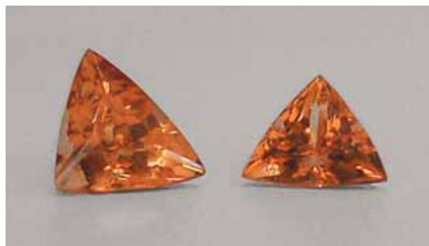
Figure 35. These two samples of synthetic corundum (2.03 and 1.18 ct) were sold in Minas Gerais, Brazil, as Imperial topaz. Photo by M. Macrì.
