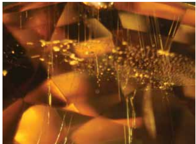
Figure 10. One of the danburites also contained elongate growth tubes. Photomicrograph by Hpone Phy Kan-Nyunt; magnified 20×.
