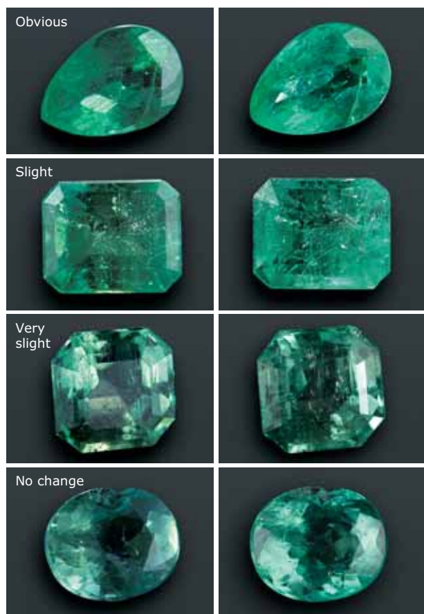
Figure 3. Changes in emerald appearance after durability tests (before, left; after, right) were divided into four categories: obvious (no. 4706, 0.79 ct, ultrasonic cleaning in water); slight (no. 4633, 1.09 ct, ultrasonic cleaning in BCR); very slight (no. 4936, 2.95 ct, steam cleaning); and no observed changes (no. 4757, 0.46 ct, ethanol and acetone cleaning).
