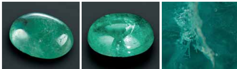
Figure 6. This 3.57 ct emerald filled with paraffin oil (no. 4747; left) showed obvious changes due to time alone (center). Feathers, especially to right of center, were observed as more open (right, magnified 40 \times ).
