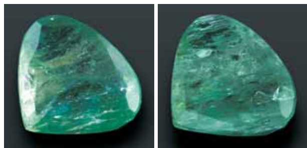
Figure 17. This 1.00 ct emerald, filled with a mixture of Canada balsam and cedarwood oil, looks yellowish in fissures after filling (no. 4773; left), but much of this color went away (along with the filler) after soaking in ethanol (right).
