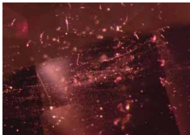
Figure 33. These curved particle trails and straight/kinked hollow tubes identified the sample in figure 32 as a flame-fusion synthetic. Photomicrograph by M. S. Krzemnicki, © SSEF; magnified 30×.
