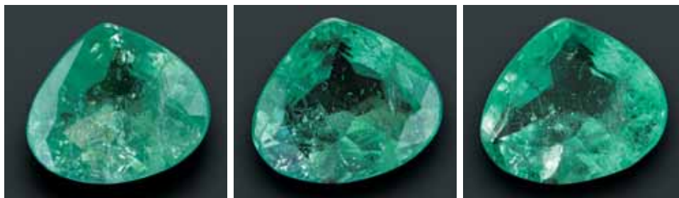
Figure 10. This 0.95 ct emerald (no. 4807; left) was filled with unhardened Opticon (center) and showed an obvious change, in the form of more prominent feathers (right), after a year in a desiccation chamber.
