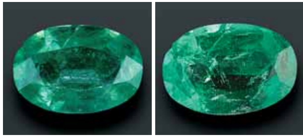
Figure 14. The fissures in this 0.74 ct emerald filled with Araldite 6010 (no. 4600; left, after filling) had been partly emptied out following 30 minutes of ultrasonic cleaning in BCR, an obvious change (right).
