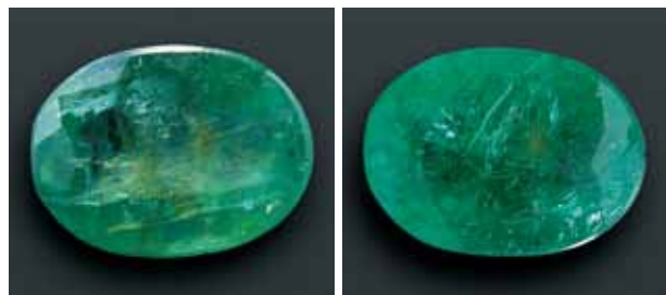
Figure 2. This emerald, filled with a mixture of cedar-wood oil and Canada balsam (no. 4728; left), had an obvious change due to ultrasonic cleaning in BCR (right). However, the appearance of the emerald in these photos, along with all the emerald photos, was influenced by changes in the choice of photos, intensity of light, film, and processing choices by the different photographers. Therefore, the fissures visible parallel to the long axis of the emerald are not as evident in the right image, and the emerald's color looks different.
