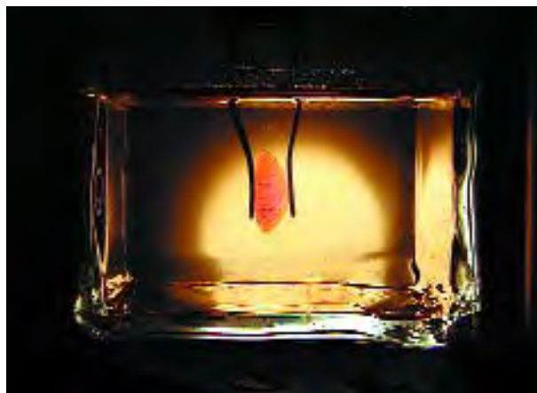
Figure 32. This Be-diffused sapphire is shown in an immersion cell filled with methylene iodide; a diffuser plate was placed between the light source and the cell. In conjunction with a horizontal microscope, this was one of the methods used to examine the stones in this study. Photo by Ken Scarratt.
