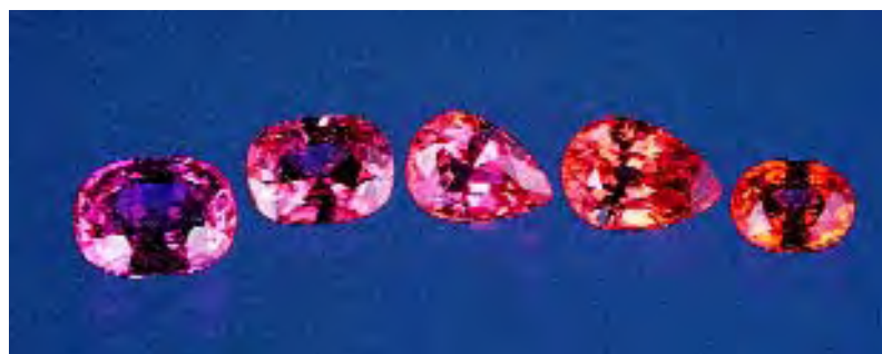
Figure 18. The depth of the Be-diffusion layer directly affects face-up color. The stone on the far left has a very shallow diffusion layer. Moving right, each stone has a progressively deeper layer, making each more orange than the last. These stones weigh 0.80–1.89 ct; photo by Maha Tannous.
