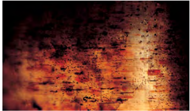
Figure 5. Oriented inclusions (probably hematite) were responsible for the chatoyancy shown by the beryls in figure 4. Photomicrograph by Jaroslav Hyrsl; magnified 9×.
