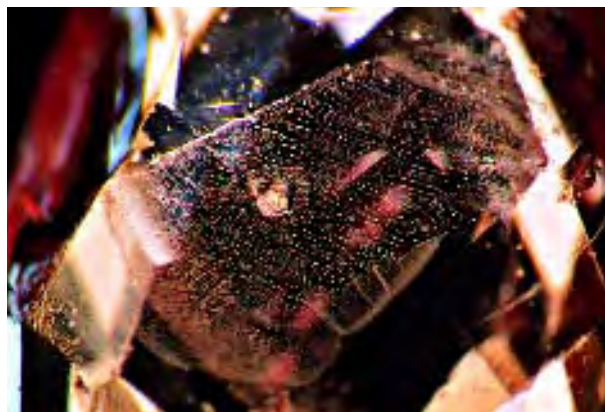
Figure 48. Healed fractures such as these were seen in many of the Be-diffused corundum samples we examined. They often appeared similar to those found in flux- or hydrothermally grown synthetic rubies and sapphires. Photomicrograph by Shane F. McClure; magnified 25 \times .
