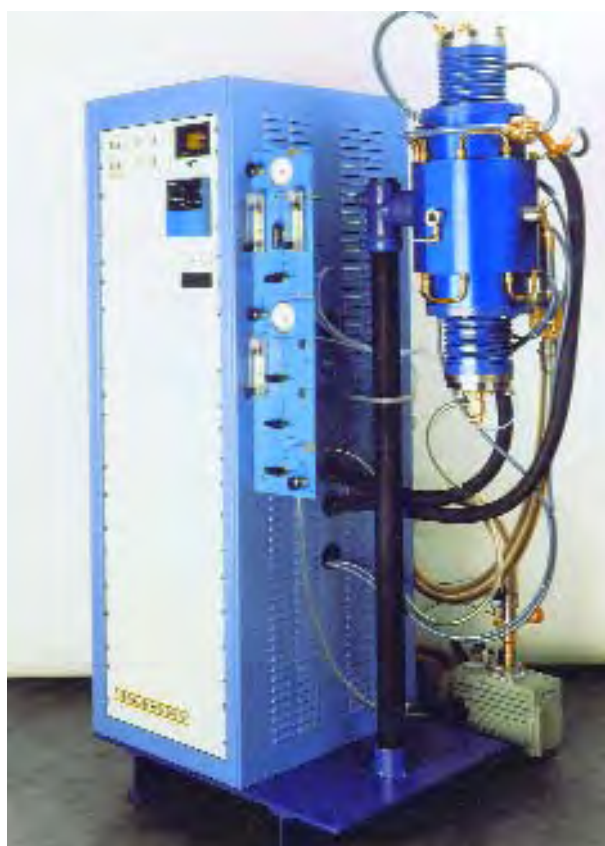
Figure 21. Most of the Be-diffusion experiments described in this article were conducted using an electrically heated furnace. Photo courtesy of Thermal Technology Inc.
