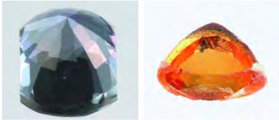
Figure 13. Many of the off-color sapphires from Songea that do not improve with standard heat treatment (left) will turn a strong orangy yellow after Be diffusion (right). This stone weighs 0.50 ct; photos by Elizabeth Schrader.
