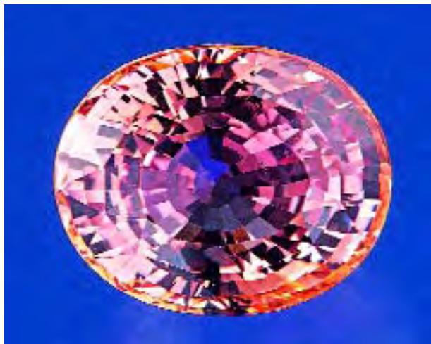
Figure 33. Not all sapphires treated with beryllium have an intense color, as this 14.38 ct Be-diffused sapphire illustrates. It has a medium tone very similar to that of some natural-color sapphires. It is interesting to note that the thin orange layer present in this stone is visible even without immersion, which is not usually the case. Photo by Maha Tannous.
