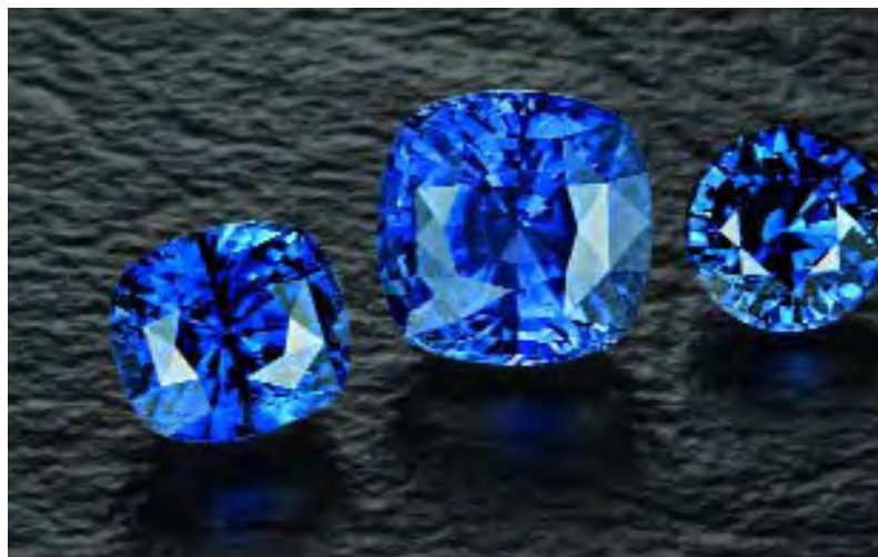
Figure 8. These magnificent blue sapphires (weighing approximately 2–4 ct) owe their color primarily to \text{Fe}^{2+}\text{-Ti}^{4+} pairs. Courtesy of Gordon Bleck; photo by Maha Tannous.
