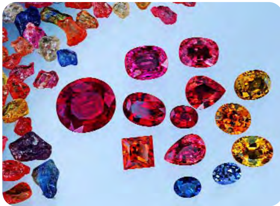
Figure 1. The beryllium diffusion process can affect many colors of corundum, including ruby and blue sapphire. The Be-diffused stones shown here range from 0.40 to 5.05 ct. Photo by Harold & Erica Van Pelt.
