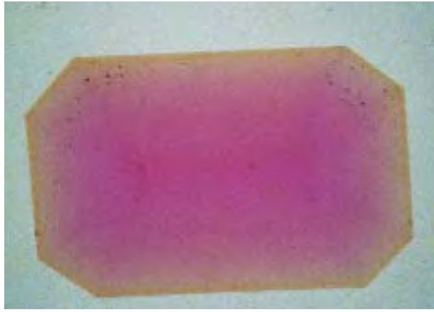
Figure 2. Most of the Be-diffused stones seen early on, particularly in the pink-orange color range, showed distinct yellow-to-orange surface-conformal layers when viewed in immersion. Photomicrograph by Shane F. McClure; magnified 10 \times .
