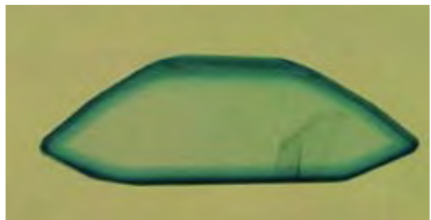
Figure 16. A dark blue color layer is formed near the surface when Ti is diffused into sapphire. This 1.3-mm-thick section was sawn from a 1.45 ct stone, and shows a Ti diffusion-induced layer of blue color that is 0.4 mm deep. Photo by Shane F. McClure; immersion.
