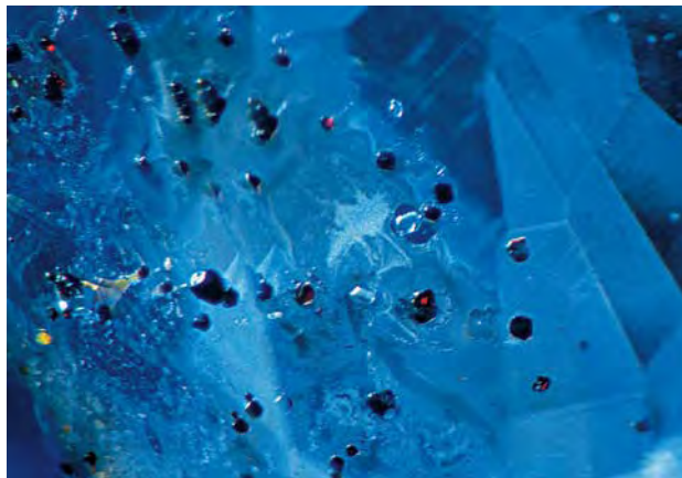
Figure 25. In contrast to their brownish yellow color in the sapphire shown in figure 24, pyrochlore inclusions in blue sapphire typically are dark brownish red. Photomicrograph by John I. Koivula; magnified 20×.
