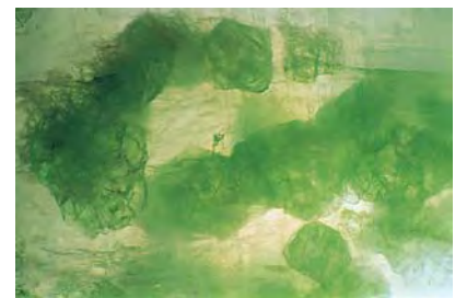
Figure 6. The rounded appearance and cracked texture of the chrome diopside inclusions in their orthoclase host suggest that the inclusions are protogenetic. Magnified 5×.
