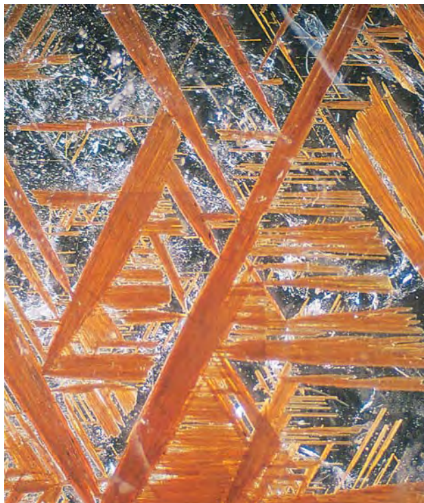
Figure 15. With magnification (here 5×), the complex branching growth of the twinned rutile structure is seen in detail. In darkfield illumination, the red-brown color of the rutile is also apparent. Photomicrograph by John I. Koivula.
