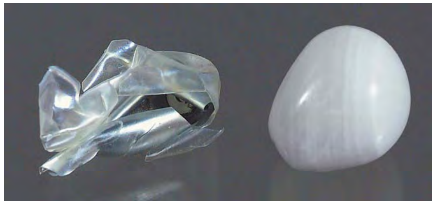
Figure 15. The coating removed from the imitation "shell" pearl was found to consist of two types of layers (left): external transparent colorless layers and internal opaque light gray metallic layers. Gemological testing identified the bead nucleus (right) as calcite.
