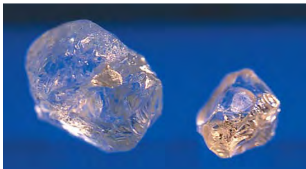
Figure 32. Represented as diamond rough in Brazil, these imitations consist of topaz (23.57 ct, left) and cubic zirconia (8.71 ct, right) to which small fragments of diamond have been attached in discrete crevices. The seller could then place a diamond probe on the small piece of diamond to “prove” that the entire piece was “natural.” Photo by H. A. Hänni.
