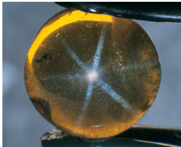
Figure 8. The almost-perfect six-rayed star in this transparent 3.29 ct chrysoberyl was found to be manufactured. Photomicrograph by Shane F. McClure; magnified 10×.
