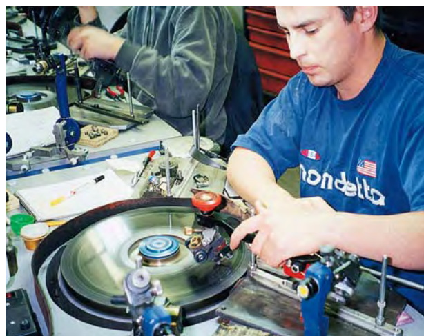
Figure 4. Shane Fox, one of about 20 cutters presently working at the Sirius Diamonds factory in Yellowknife, is shown faceting a round brilliant. The company currently cuts 500–600 carats of rough Ekati diamonds per month. Photo by K. A. Mychaluk.
