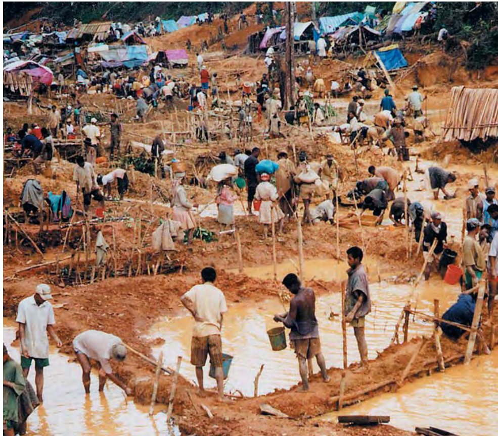
Figure 21. In a rush to stake their claims, tens of thousands of miners have journeyed to the Andilamena area. The rubies are mined by simple methods from a layer of gravel that typically lies 2–3 m below the surface. Photo by Rakotosaona Nirina.
