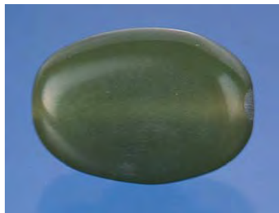
Figure 7. This 10×7×3.5 mm bead, which looks like nephrite jade, was identified as dyed gibbsite.
