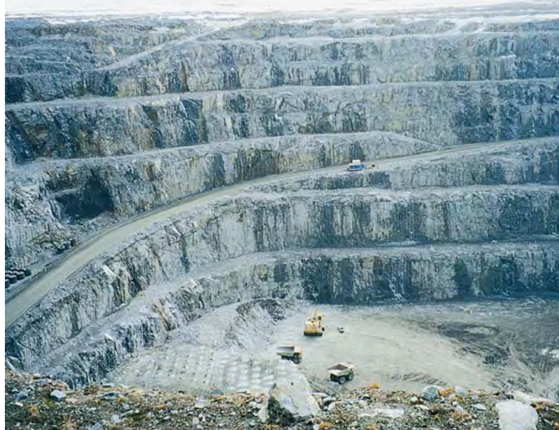
Figure 2. The Panda pit at the Ekati mine, currently 150 m deep, is now at half its projected open-pit depth of 300 m. The predominant rocks in the photo are granitic country rocks that surround the diamond-bearing kimberlite (not visible). The rectangular area in the lower left corner of the pit has been drilled in preparation for blasting. The ore trucks are designed to haul 240 tons of rock. Photo taken on May 27, 2001, by K. A. Mychaluk.
