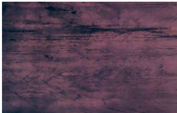
Figure 10. Numerous fibrous inclusions are present in the cat's-eye amethyst shown in figure 9, and are oriented perpendicular to subtle color zoning. Note also the smaller fibrous inclusions oriented at approximately 45° to the main direction. Photo by Jaroslav Hyrsl; width of view 5.4 mm.
