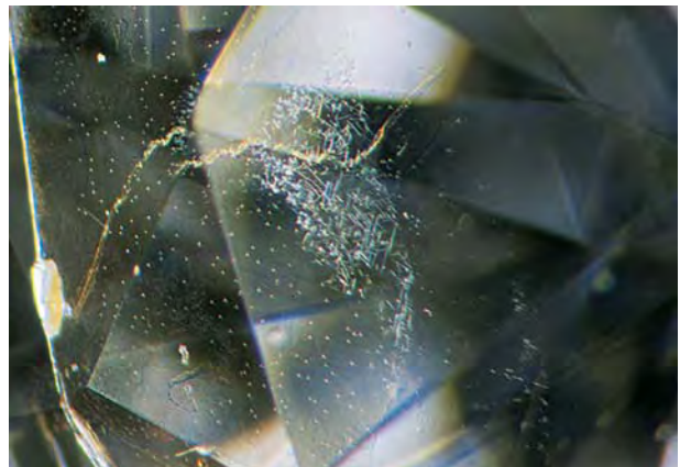
Figure 9. In addition to a group of intersecting colorless crystals, this break in a new Oved filled diamond shows a pattern of gas bubbles that are relatively evenly dispersed. Photomicrograph by John I. Koivula; magnified 40×.
