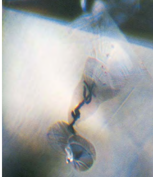
Figure 18. The internal channels became very difficult to see when light was reflected off the host feather, as is the case with the top half of the feather shown here. Note, though, that the widening of the feather is clearly visible. Photomicrograph by Shane F. McClure; magnified 40 \times .
