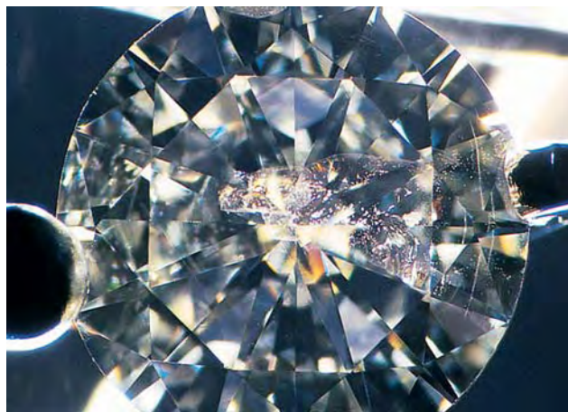
Figure 10. Four of the eight Oved diamonds tested showed minor damage after retipping. The photo on the left shows one of these diamonds (1.03 ct) before retipping. After the procedure (right), the glass-filled fractures showed a loss of filler that appears as reflective areas within the fractures. Photos by John I. Koivula (left) and Shane F. McClure (right).
