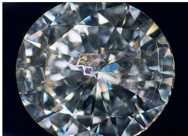
Figure 10. Four of the eight Oved diamonds tested showed minor damage after retipping. The photo on the left shows one of these diamonds (1.03 ct) before retipping. After the procedure (right), the glass-filled fractures showed a loss of filler that appears as reflective areas within the fractures. Photos by John I. Koivula (left) and Shane F. McClure (right).
