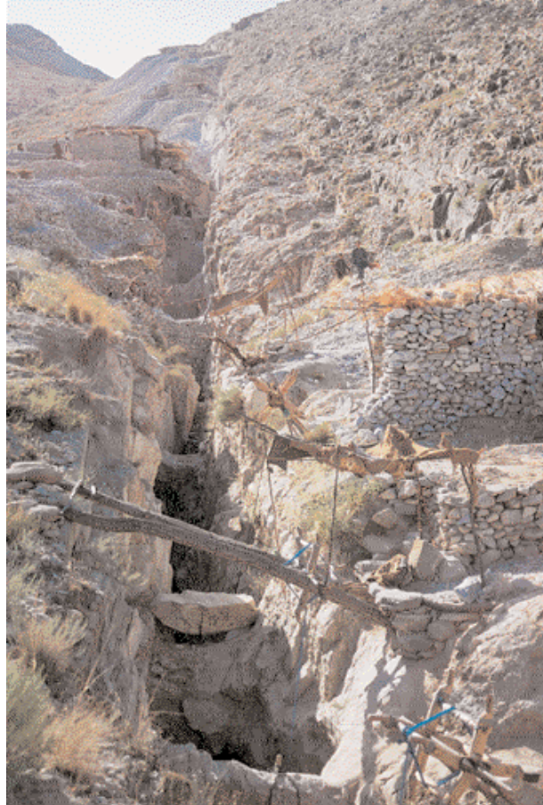
Figure 7. In 1996, the miners started new trenches on the western end of the Jegdalek deposit. These trenches follow the veins in an east-to-west direction. Photo by Gary Bowersox.
