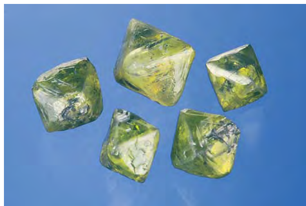
Figure 10. These five diamond crystals (1.90 to 4.45 ct) changed from brown to greenish yellow due to HPHT treatment by Novatek. Photos by Elizabeth Schrader
