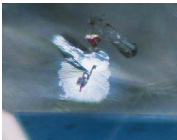
Figure 14. It appears that the channels, shown here in the center of the bright area, serve to widen the feathers, thus allowing penetration of the acids used to bleach the inclusions. This is evidenced by the higher visibility of the areas immediately surrounding the channels. Photomicrograph by Vincent Cracco; magnified 63 \times .
