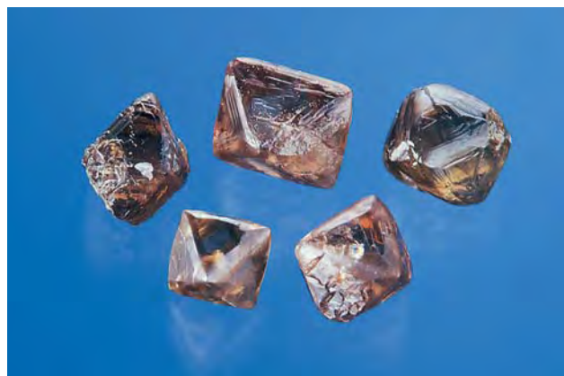
Figure 10. These five diamond crystals (1.90 to 4.45 ct) changed from brown to greenish yellow due to HPHT treatment by Novatek. Photos by Elizabeth Schrader
