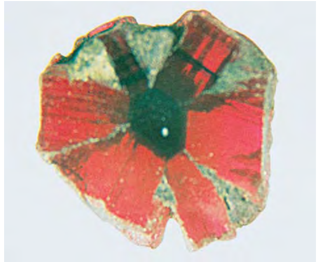
Figure 15. This trapiche ruby from Mong Hsu, Myanmar, consists of a dark violet, almost black core, six white arms that widen toward the outer edge of the crystal, and six trapezoidal ruby sectors. In some of these transparent ruby sectors, a distinct red and dark violet color zoning parallel to dipyrmaid growth planes was observed with magnification. The sample measures about 5.5 × 6 mm. Photo by K. Schmetzer.
