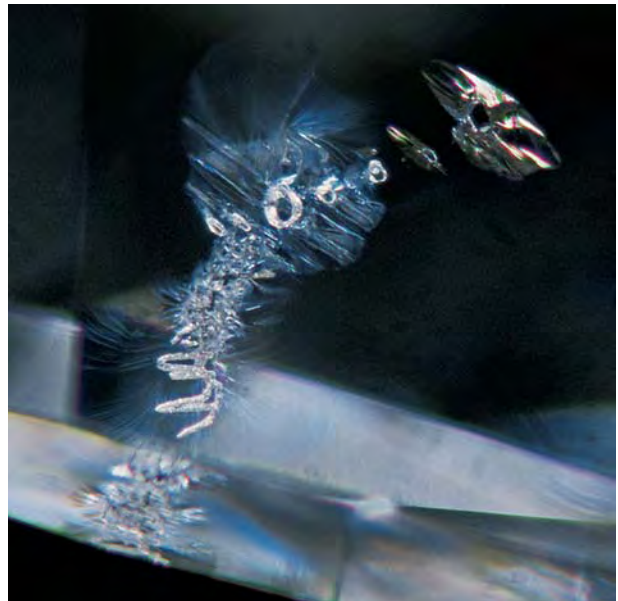
Figure 8. The wormhole-like channels took on a variety of appearances in these treated diamonds. These channels lead from the feather on the surface to a group of crystals and accompanying feathers. Note that the large crystal on the upper right has not been treated. Photomicrograph by Vincent Cracco; magnified 63×.
