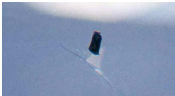
Figure 12. This cavity, which appears black in reflected light, was not present before the diamond (sample no. 4) was treated, which suggests that there is some risk involved in using this new technique. Photomicrograph by Shane F. McClure; magnified 40 \times .
