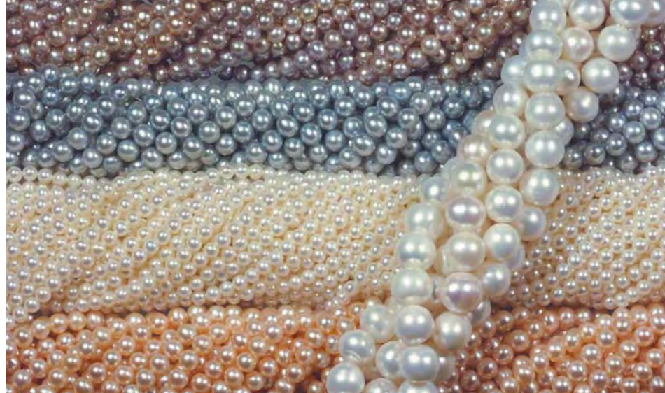
Figure 7. These round Chinese freshwater cultured pearls are representative of the samples examined for this study. The largest white FWCPs shown are 10–11 mm in diameter. Photo by Elizabeth Schrader.
