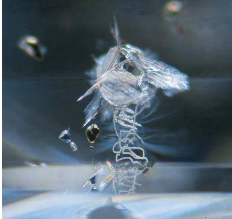
Figure 1. The appearance within feathers of unnatural, irregular, wormhole-like channels provided the first clue that a new laser treatment had entered the market. Photomicrograph by Vincent Cracco; magnified 63×.
