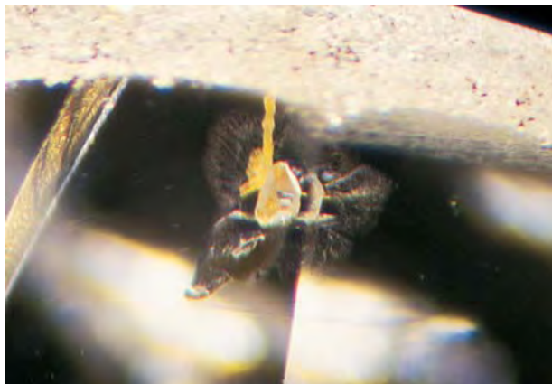
Figure 7. This laser drill hole was filled by glass during the Oved treatment process. Photomicrograph by Shane F. McClure; magnified 40×.
