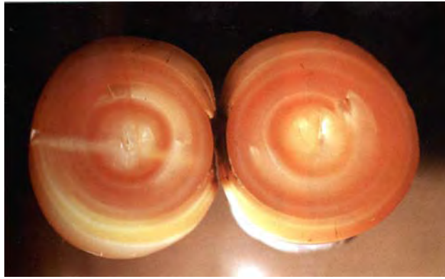
Figure 15. The concentric growth structures in these 12 mm (left) and 8.5 mm (right) Chinese FWCPs that have been sawn in two are entirely normal for tissue-nucleated freshwater cultured pearls. No indications of a solid nucleus of any type were seen. Photos by Kenneth Scarratt.
