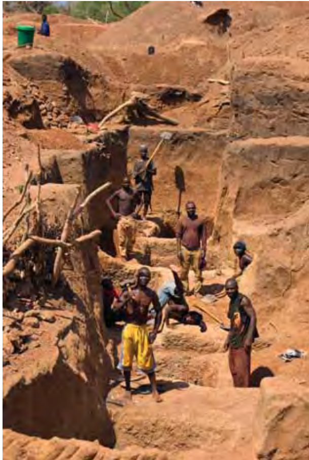
Figure 11. Most of the Cu-bearing tourmaline recovered so far from the Mavuco area has come from artisanal miners. Working in small groups, they use picks and shovels to dig through the laterite overburden in search of the gem-bearing layer. Photo by B. M. Laurs.
