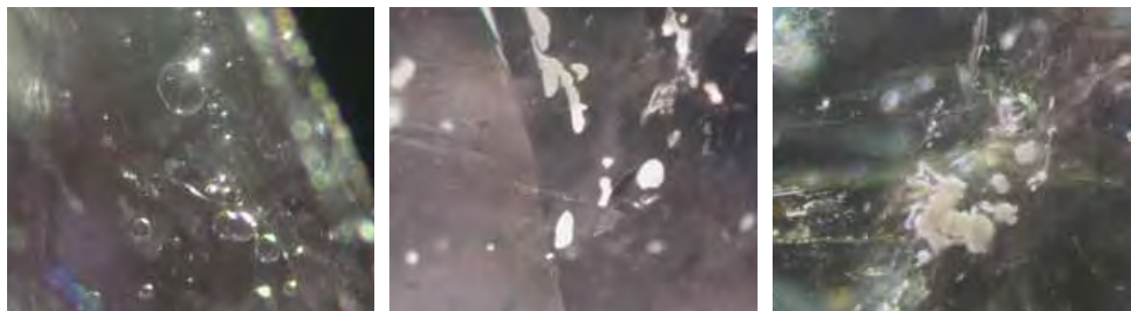
Figure 32. The lead glass-filled fissures showed rounded (left) and flattened (center) gas bubbles, the latter often highly reflective, an important identifying feature for this treatment. Some whitish crystallites were also seen in a few cavities (right). Photomicrographs by G. Choudhary; magnified 45× (left and center) and 35× (right).
