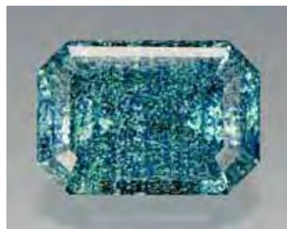
Figure 17. This 0.91 ct octagonal step cut represents an unusual color for flame-fusion synthetic sapphire.
