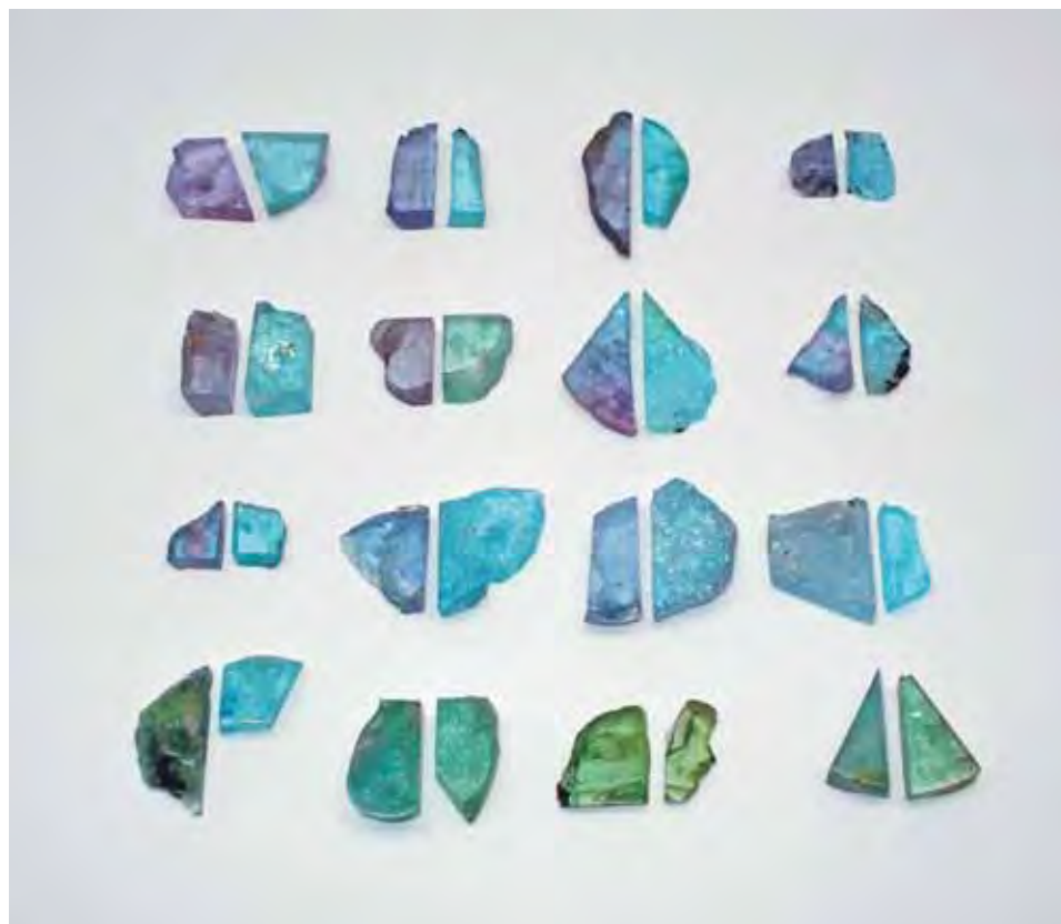
Figure 22. Each pair of parallel-polished plates shown here (0.98–7.15 ct) was sliced from the same piece of rough. The segments on the left in each pair are unheated, and those on the right were heated to 530°C for three hours. These slices formed part of the study suite of samples examined before and after heating. Gift of Barker & Co. and Pala International, GIA Collection nos. 37519–37540; photo by J. C. Zwaan.
