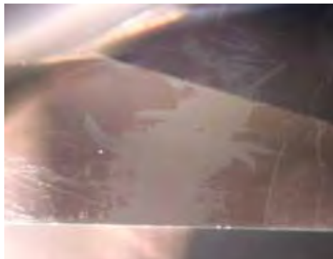
Figure 6. The diamond on the left proved to be a cape stone with a pink coating on the girdle. Note the iridescence and irregular surface features. At right, scratches in the pink coating on this stone are also indicative of this treatment. Photomicrographs by Andrew Quinlan, left (magnified 63×), and Wuyi Wang, right (100×).
