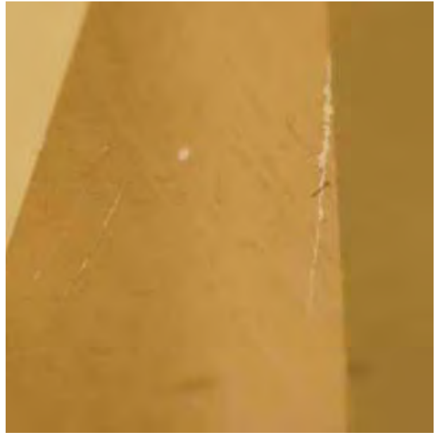
Figure 5. Colorless spots, dark stains, and scratches occurred randomly on some coated facets. Photomicrograph by W. Wang; magnified 112 \times .
