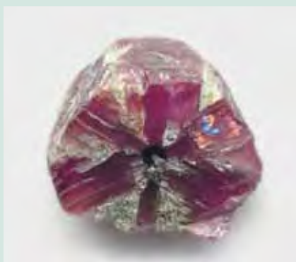
Figure A-2. In these trapiche rubies from Mong Hsu, skeletal growth is responsible for the “star.” On the left (5.7 × 5.0 mm), typical skeletal growth formed a simple star; on the right (8.2 × 6.6 mm), very strongly developed skeletal growth resulted in a star motif of the gemmy sectors that is created by triangular opaque skeletal arms. Photos by T. Hainschwang.
