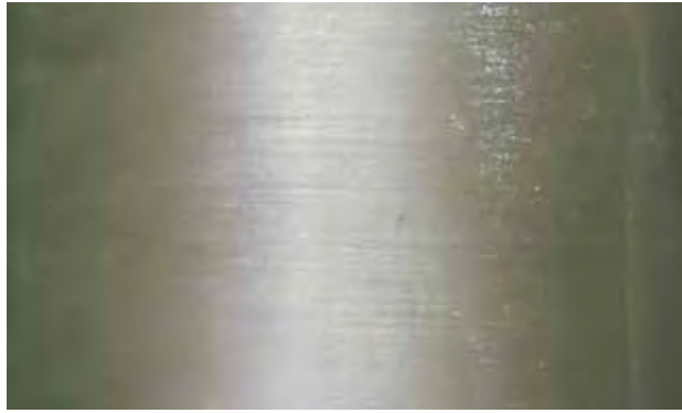
Figure 42. Numerous extremely thin parallel channels or platelets are the cause of the chatoyancy in the cat's-eye prehnite. Small fissures can also be seen near the right side of this view. Photomicrograph by S. Singbamroong, © Dubai Gemstone Laboratory; magnified 20 \times .
