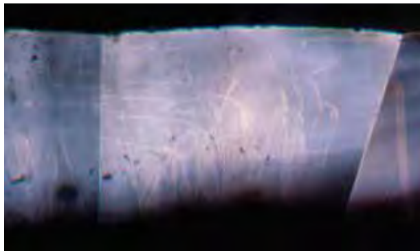
Figure 29. Scratches or other damage to a coating often make it easier to detect. Photomicrograph by S. F. McClure; magnified 35 \times .
