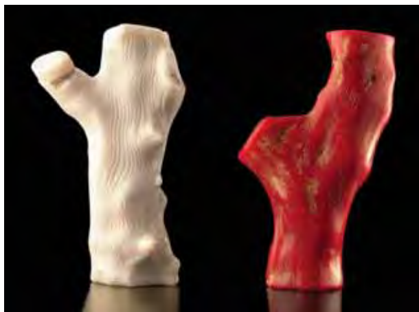
Figure 3. The coral branch on the left (67 mm) has been bleached, which is commonly performed prior to dyeing to improve the penetration of the dye and allow for a more homogeneous coloration after dyeing. The branch on the right has been dyed red. Also clearly evident in these two samples of Corallium rubrum are striations parallel to the length of the branches. The grooves are canals that the coral polyps used to transport nutrients and are one of the most distinguishing characteristics of the coral structure. Photo by Jessica Arditi.
