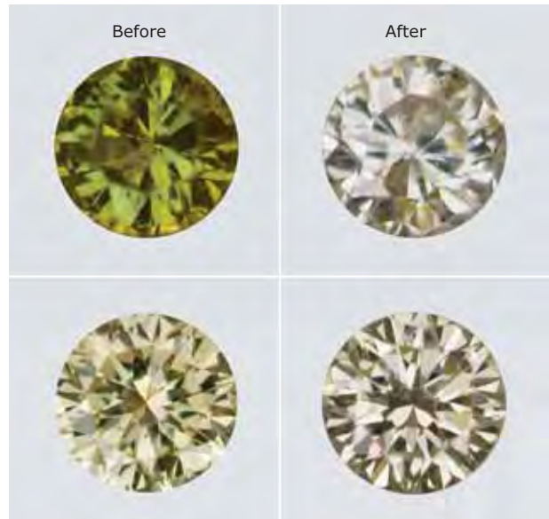
Figure 23. The coatings were removed from these diamonds (0.01–0.02 ct) by immersion in undiluted Clorox bleach for 48 hours. Top—a Fancy Deep green-yellow diamond (left) received a color grade of N on the D-Z color scale (right). Bottom—a Fancy Light yellow diamond (left) was graded V color (right). Photos by Robison McMurtry.
