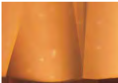
Figure 28. Reflected light (left) and transmitted light (right) can both be used to see the small rounded uncoated areas on these diamonds. Photomicrographs by John I. Koivula (left, 25 \times ) and S. F. McClure (right, 23 \times ).
