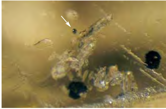
Figure 47. Also present in one of the dravite samples were colorless low-relief crystals (identified as an amphibole by Raman analysis), black disk-shaped crystals (probably graphite), and a minute rounded crystal with a brassy luster (probably pyrite; see arrow). The latter two inclusions were too deep in the stone for identification by Raman analysis. The birefringence of the amphibole inclusions is shown in the photo on the right, taken in cross-polarized light. Photomicrographs by J. I. Koivula; magnified 15 \times .
