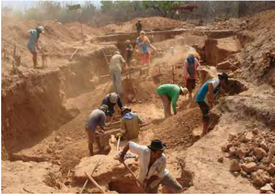
Figure 9. Workers use hand tools and dry sieves to mine for opals at this alluvial deposit near Pedro II in Piauí, Brazil. Courtesy of Opalas Pedro II.
