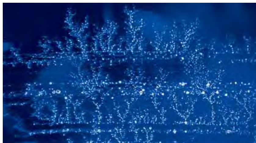
Figure 17. The rows of unusual tree-like inclusions in this sapphire probably formed through exsolution as a result of the heat-treatment process. Their composition is unknown. Magnified 10 \times .
