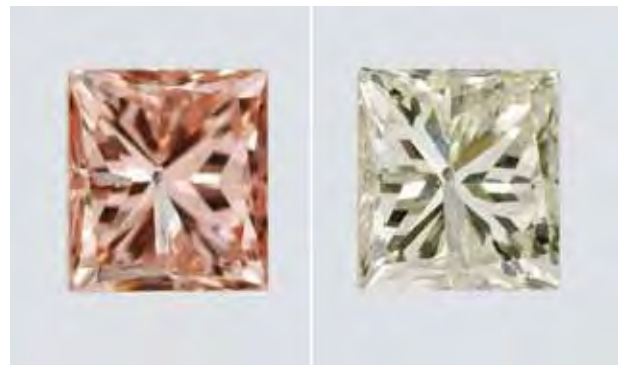
Figure 22. When this pink-coated diamond (0.50 ct) was boiled in sulfuric acid for 30 minutes, the coating was completely removed and the sample regained its original light yellow coloration. Photos by Jian Xin (Jae) Liao.
