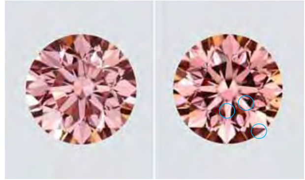
Figure 20. These images show that the jewelry repair tests had some effect on this 0.40 ct pink-coated diamond's apparent color. While the stone was graded Fancy Intense pink both before and after the tests, following rhodium plating approximately 10% of the surface showed evidence of damage in the form of uneven color distribution (see, e.g., circled areas). Photos by Jian Xin (Jae) Liao (left) and Robison McMurtry (right).
