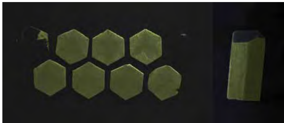
Figure 8. Chalky yellow short-wave UV fluorescence was shown by the slices and crystals of trapiche tourmaline. However, the faces of the trigonal pyramid were inert. Photos by T. Hainschwang (samples TH 682–6810; ~8.4 mm in diameter).
