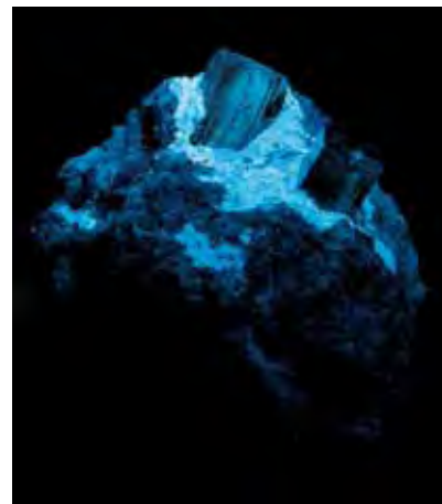
Figure 14. The extent of the glue used to affix the emerald crystals in the matrix became very apparent when the specimen was exposed to long-wave UV radiation. Notice how visible the writing in one of the crystals is.
