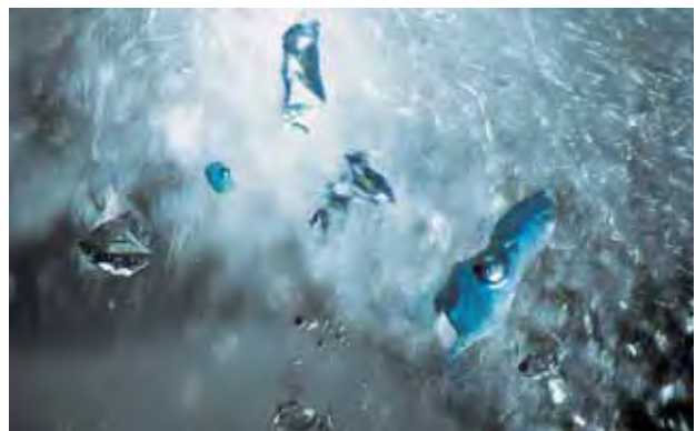
Figure 20. A few of the smaller blue fluid inclusions in the Brazilian quartz had a well-developed negative crystal form. Photomicrograph by J. I. Koivula for microWorld of Gems ; magnified 30 \times .
