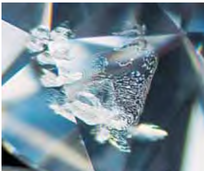
Figure 5. These fingerprint-like inclusions seen in two natural-color type IIa colorless diamonds show a channel structure that is remarkably similar to the “fingerprints” commonly found in ruby and sapphire. Magnified 45× (left), 30× (right).
