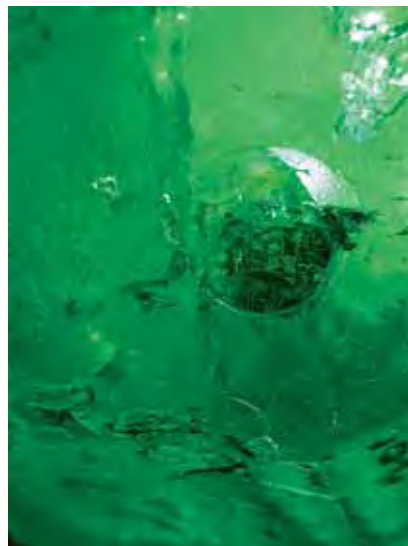
Figure 15. This view through the termination of one of the emerald crystals in figure 13 reveals that a hole had been drilled down the center from the bottom without breaking the surface of the termination. Magnified 10 \times .
