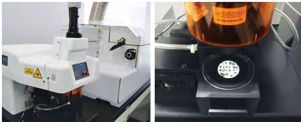
Figure 10. The LA-ICP-MS system used in this study is shown on the left, with the laser ablation unit in the left foreground and the ICP-MS instrument behind it. The photo on the right is a close-up view of samples in the ablation chamber. Photos by Masaaki Kobayashi (left) and A. Abduriyim (right).
