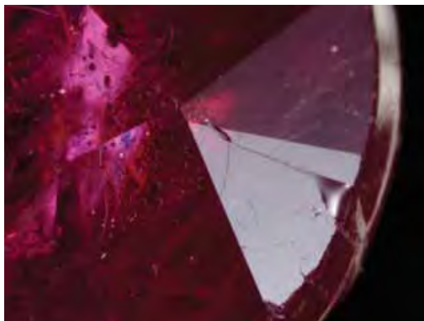
Figure 21. Heating at 700°C for only a few minutes caused the lead-based glass in larger cavities to start to flow. Photomicrograph by C. P. Smith; magnified 24×.
