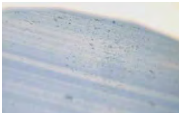
Figure 27. With immersion in methylene iodide and diffuse illumination, straight and parallel blue color zones are clearly visible across the color plane in the sapphire. Photomicrograph by G. Choudhary; magnified 35x.
