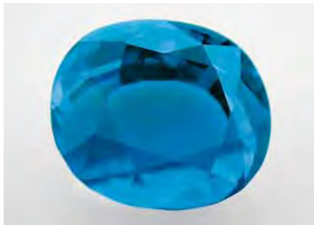
Figure 25. Although this 11.29 ct sapphire appears an attractive, uniform blue when viewed face up, its color is actually restricted to a narrow zone on the pavilion. Photo by G. Choudhary.
