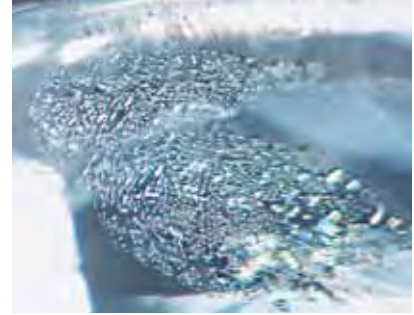
Figure 4. A fingerprint-like inclusion seen recently in this 0.64 ct natural-color Light blue diamond actually consists of groups of many tiny crystals. Magnified 45×.
