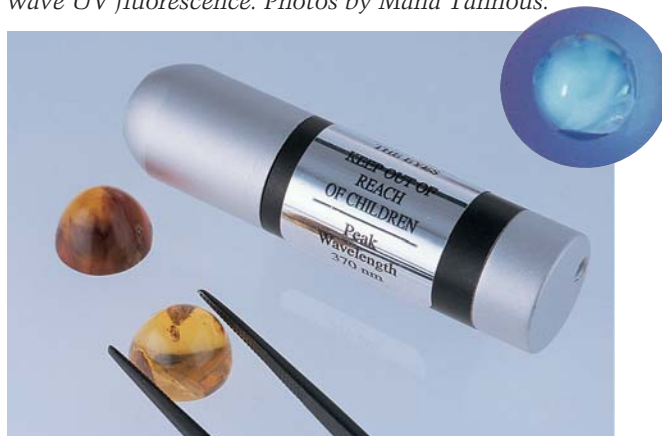
Figure 12. The lipstick-size (5.5 × 1.5 cm) long-wave portable ultraviolet lamp from Nebula, Redwood City, California, is one of the most durable UV lamps introduced in the last few years. Inset: Natural amber generally fluoresces blue under long-wave UV fluorescence. Photos by Maha Tannous.
