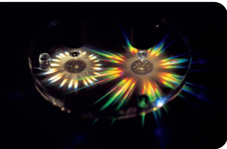
Figure 22. The narrow white flares from a faceted diamond (left) readily separate it from the broad spectral flashes of a faceted synthetic moissanite (right)—illustrating the differences in dispersion—when the two round brilliants are submerged in water and illuminated from above through a pinhole with a focused light source. This concept of optical dispersion is the essence of the Hodgkinson “Visual Optics” method. Photo by Alan Hodgkinson.
