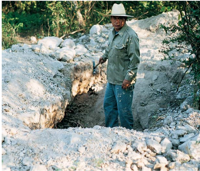
Figure 18. An alluvial deposit of high-quality black spinel was found in January 2000 in Nayarit State, Mexico. Arturo Hernandez, who discovered the deposit, is standing in an exploratory pit in La Vieja creek that yielded approximately 5 kg of spinel from 5 m 3 of alluvium. Photo by William Rohtert.
