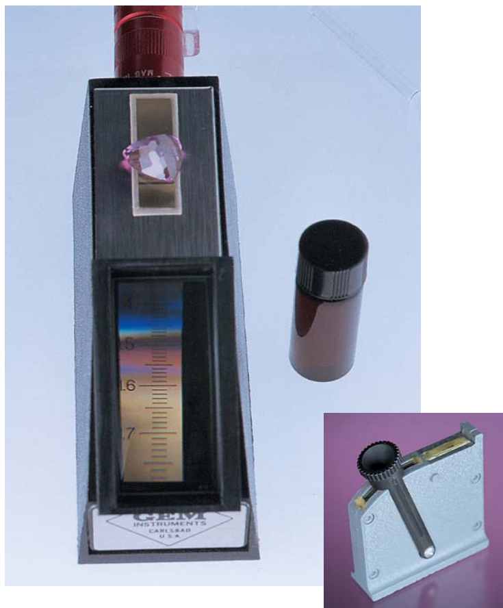
Figure 20. Among the portable refractometers currently available is the GIA Gem Instruments Duplex III (shown with a 4.95 ct spinel). The inset shows the GIA Gem Instruments refractometer designed by Robert Shipley Jr. that was introduced in 1949. At 5.2 × 4.8 cm, it is still considered one of the most durable and portable refractometers ever made (E. Gübelin, pers. comm., 2002). Photos by Maha Tannous.
