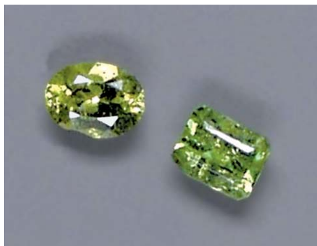
Figure 22. These two 0.26 ct vesuvianites came from a small parcel of faceted material purchased in Madagascar. Their yellowish green color is attributed to Cr 3+ . Photo by Franzisca Imfeld.
