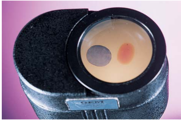
Figure 23. Diffusion detectors can be very useful for detecting surface-diffused gems, even when water or oil is used as the immersion medium rather than methylene iodide. Surface-diffused sapphires (here, a blue sapphire on the left showing blue color concentrations along the facet junctions, next to an orangy pink sapphire with a distinctive rim of surface color) continue to pose identification challenges for gemologists. Photo by Maha Tannous.
