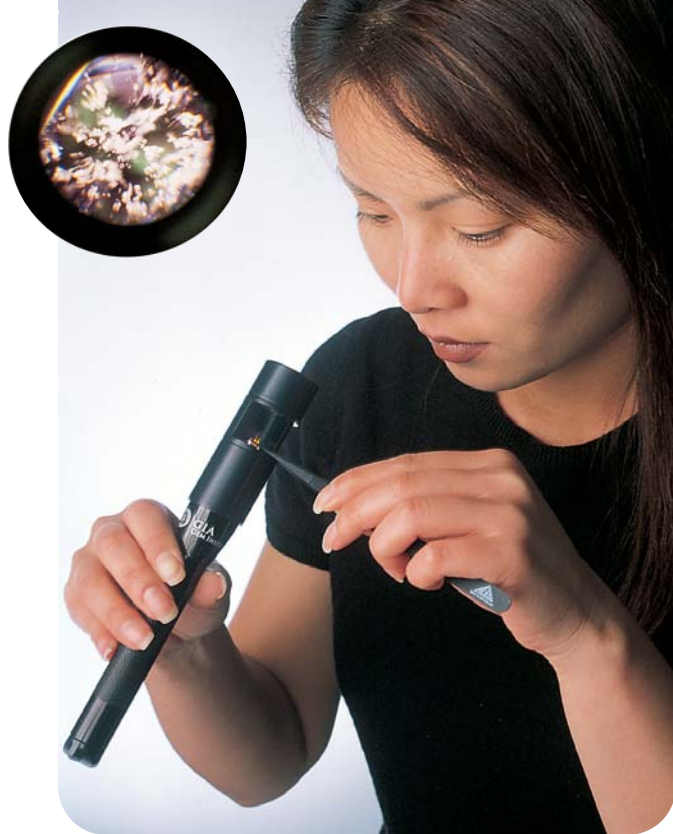
Figure 9. Proper use of the darkfield loupe (here, by GIA Gem Instruments) requires practice holding the gem in one hand and the loupe and flashlight together in the other at a distance of about one to two inches (3–5 cm) from the eye. In the inset, a typical inclusion scene of negative crystals is readily visible with a darkfield loupe in this 4.95 ct lavender spinel from Sri Lanka. Photo by Maha Tannous; inset by Edward W. Boehm.
