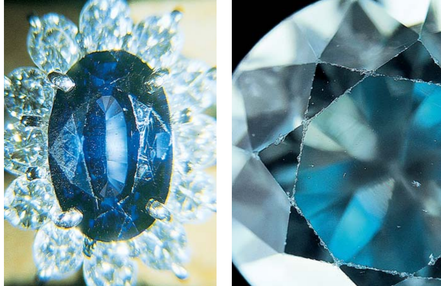
Figure 4. Surface abrasions can be a key indicator of hardness, but they do not always represent a soft stone. For example, the sapphire on the left shows a significant amount of surface abrasion, like the (much softer) zircon on the right. Abrasion and scratches are related to the amount of wear and tear, as well as to a stone's hardness. Photos by Nicholas DelRe (left) and Tino Hammid (right); © GIA.
