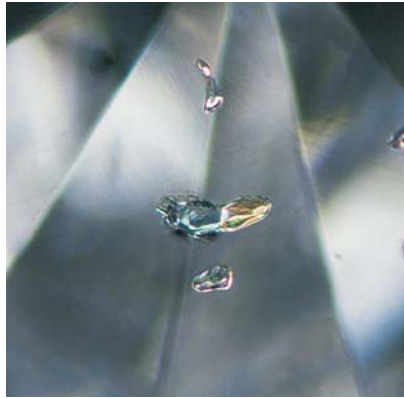
Figure 2. The “bicolored” inclusion in this diamond actually consists of a bluish green omphacitic pyroxene (left) and a brownish yellow almandine-pyrope garnet (right) that are in direct contact. Stress fractures and graphitization developed around the pyroxene, but not the garnet. Magnified 45×.
