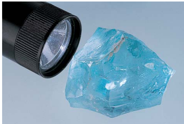
Figure 10. The gas bubbles in this glass imitation of aquamarine (4.0 × 4.0 cm) are easily visible with the aid of a 10× loupe and a powerful portable light source such as the Sure Fire light by Laser Products of Fountain Valley, California. Photo by Maha Tannous.
