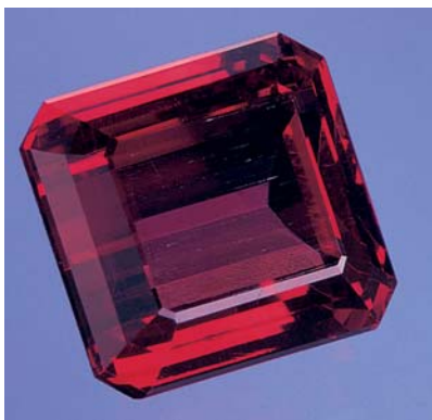
Figure 7. This 8.16 ct orange-red emerald cut is only the second example of gem-quality genthelvite that the laboratory has seen.
