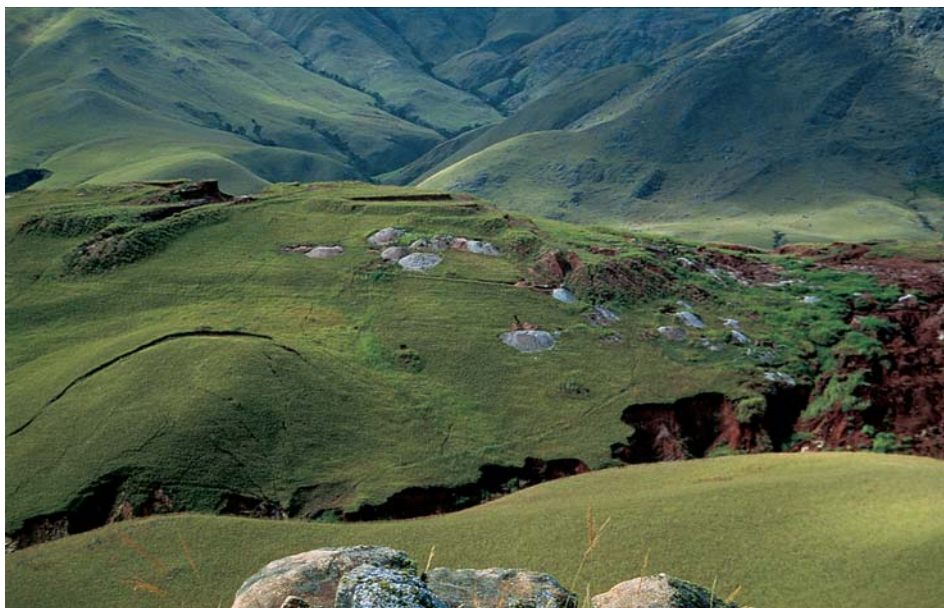
Figure 5. The historic Anjanabonoina mining area is situated on a low hill that contains several pegmatites and associated eluvial deposits. This view of the northeastern side shows a portion of the eluvial workings (right), as well as several white dump piles from pegmatite exploration activities in 1995–1996. The lower dump in the center marks the entrance to a 185-m-long prospect tunnel, and those further up the hill show the location of exploratory shafts (up to 45 m deep). Photo by Federico Pezzotta, January 1996.
