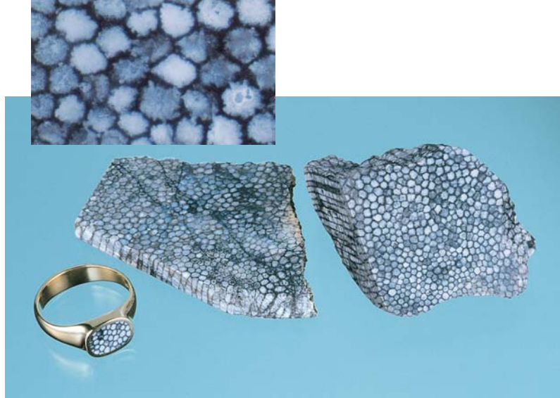
Figure 7. “Stingray” coral is a new gem material from Alaska. Distinctive patterns are created by its cellular structure (see inset). The polished slab in the center measures 6.1 × 3.6 cm; photo by Maha Tannous. Inset photomicrograph by John I. Koivula; magnified 10×.
