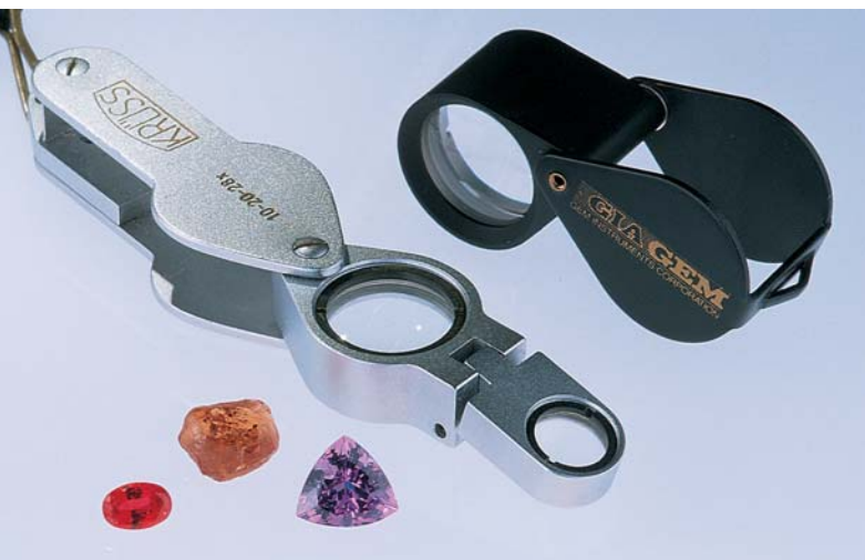
Figure 7. The loupe is a gemologist's most useful and portable tool. Shown here are a GIA Gem Instruments 20.5 mm, 10× triplet corrected loupe and a 10-20-28× corrected loupe from A. Krüss Optronic (Hamburg, Germany). Photo by Maha Tannous; the pink spinel trilliant weighs 4.95 ct.
