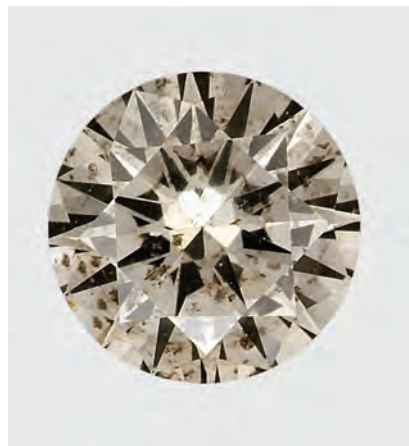
Figure 12. This 0.25 ct round brilliant with L color and I 1 clarity proved to be a type IIb CVD synthetic diamond.
