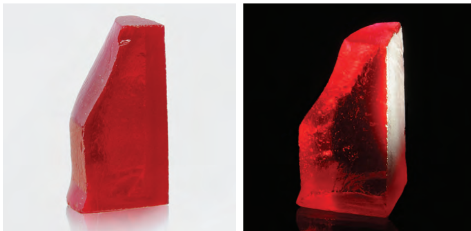
Figure 39. The 9.27 g pulled synthetic spinel is a “true” synthetic, with the bulk chemical composition and atomic structure of nominal spinel. The specimen is shown in D65 daylight-equivalent light (left) and in incandescent light, which accentuates its red color (right). Photos by O. Segura.
