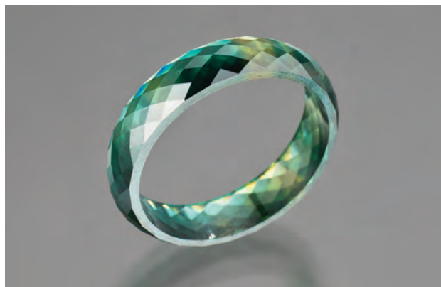
Figure 37. This ring (19 mm in diameter) was cut from a single piece of synthetic moissanite. Photo by Robert Weldon.
