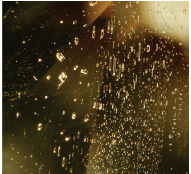
Figure 9. The 3.38 ct triangular modified brilliant in figure 7 contains a plane of elongated tubules and two-phase inclusions. Photomicrograph by D. Beaton; image width 1.5 mm.
