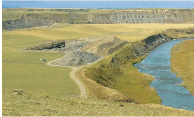
Figure 4. Outside of Korite International, only newcomer Rusty Pimm Enterprises has been successful at continuous mechanized mining for Ammolite. In this view, looking west, topsoil can be seen stockpiled on the north and west sides of the pit. Photo by K. Mychaluk.
