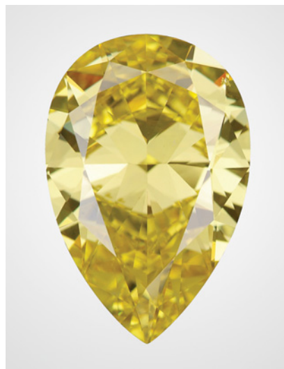
Figure 6. This 12.01 ct Fancy Vivid yellow diamond is exceptionally large for a type Ib stone and has some unusual characteristics.
