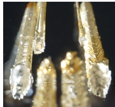
Figure 4. These etch channels display teardrop-shaped apertures, along with radiation staining and angular patterns on the body of the channel. Magnified 80\times .
