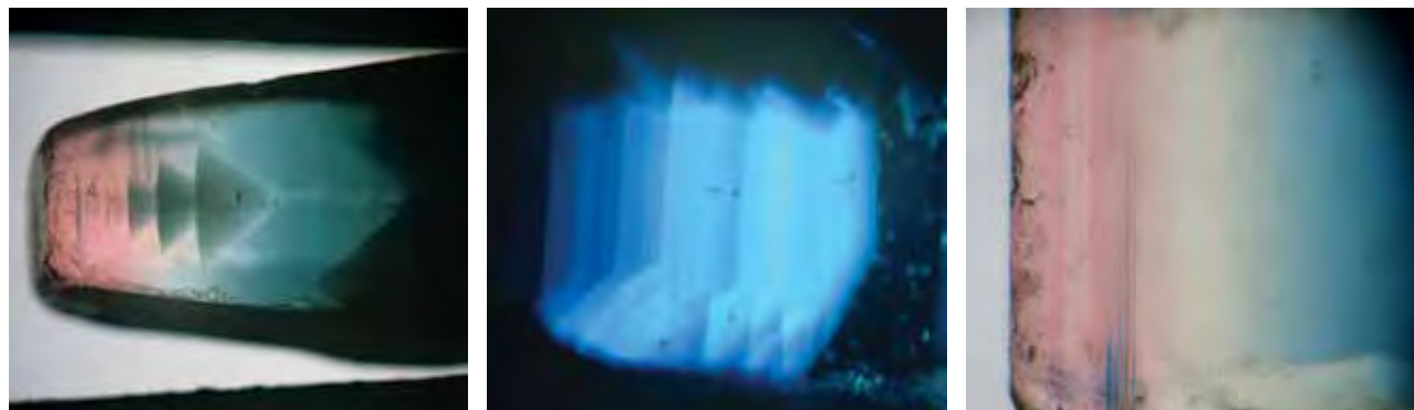
Figure 22. The color distribution of the sapphire appeared to be restricted to zones with sharp edges that followed pyramidal directions within the crystal (left and center). The purple-pink areas also displayed alternating zones of lower and higher saturation along with some blue bands, oriented parallel to the pinacoidal face (right). Photomicrographs by G. Choudhary; magnified 35× (left), 45× (center), and 60× (right).
