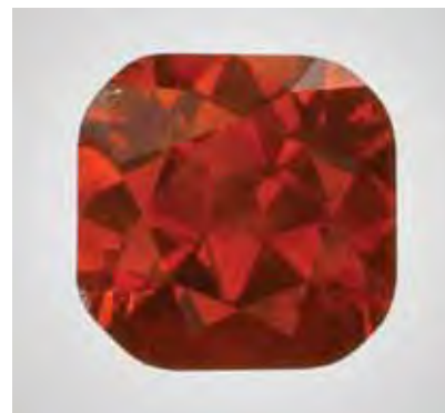
Figure 10. The unusual color of this 1.32 ct type Ib Fancy reddish orange diamond could be attributed to a specific concentration of isolated nitrogen. Reddish hues are very rare for natural type Ib diamonds.
