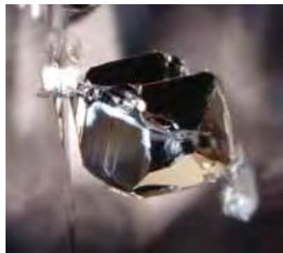
Figure 16. This large octahedron (~1.0 mm long) seen in the pinkish brown diamond is believed to be chromite. The parallel lines on its surface very likely formed simultaneously with the glide planes in the host.
