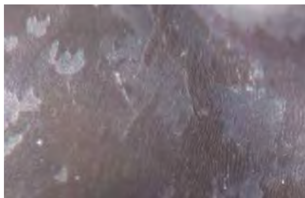
Figure 9. Large sections of the pearl surface exposed to ammonia (CCP-6) for 18 hours became discolored, with distinct light regions mixed with remnant zones of darker color. Photomicrograph by A. H. Shen; field of view 2.6 mm.
