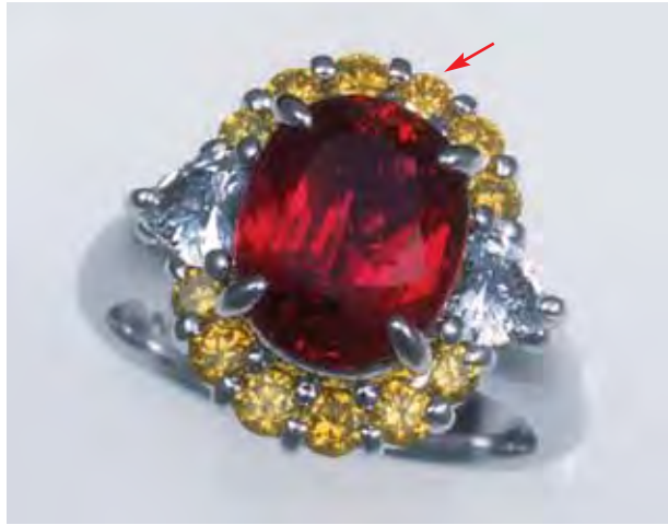
Figure 2. The GAAJ-Zenhokyo laboratory has identified yellow HPHT-grown synthetic diamond melee set with natural yellow melee in fine jewelry. In this ring, 12 melee (0.46 ct total weight) surround a 3.89 ct ruby. Only one of the 12 was natural (see arrow); all the others were synthetic. Photo by Masaaki Kobayashi.
