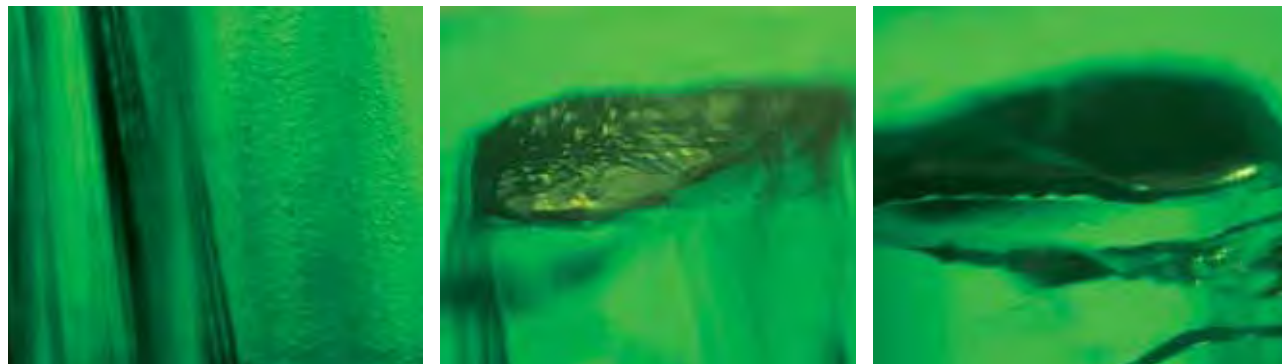
Figure 26. The included crystal displayed an etched surface along the length of its prism faces (left, magnified 80 \times ). When examined at certain angles with fiber-optic light, the pyramidal faces of the included crystal appeared bronzy, revealing complex patterns of etching and/or growth hillocks (center, magnified 65 \times ). Some angular growth features were present just below the pyramidal faces (right, magnified 80 \times ). Photomicrographs by G. Choudhary.
