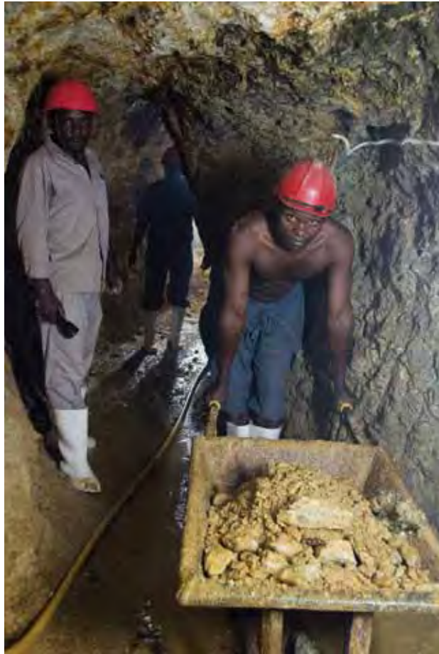
Figure 17. Ruby-bearing material from the working face of the mine is moved to the haulage shafts in wheelbarrows. Photo by B. M. Laurs.
