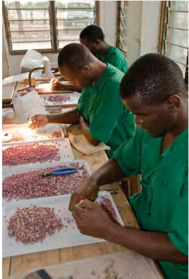
Figure 18. The corundum is carefully trimmed and sorted on site by Rockland Kenya Ltd. Photo by B. M. Laurs.
