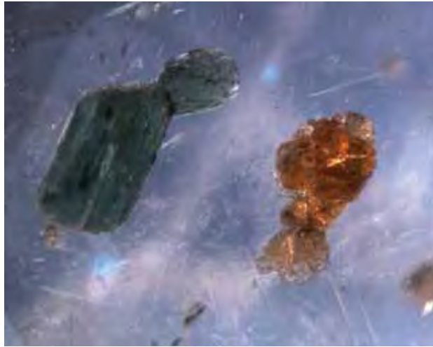
Figure 37. The green inclusions in this rose quartz from Madagascar proved to be diopside, and the orange crystalline masses were identified as grossular. Also present are some needles of epidote. Photograph by J. I. Koivula; field of view 2.7 mm.
