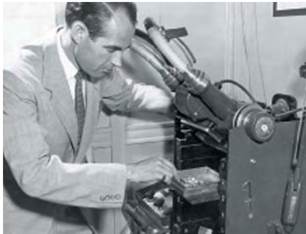
Figure 8. From its beginning, pearl testing has been a major function of the GIA laboratory. Crowningshield is shown here with the lab's "new" X-ray equipment (installed in late 1951), arranging a group of pearls on the photographic film cassette before exposing them to the X-ray beam to produce the radiograph that will determine if they are natural or cultured.
