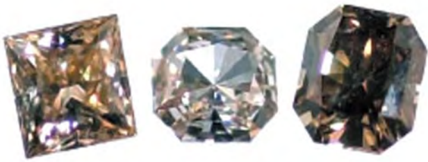
Figure 33. These three laboratory-grown diamonds (weighing 0.28, 0.14, and 0.31 ct from left to right) were produced by chemical vapor deposition. Courtesy of Apollo Diamond Inc.; photo by Elizabeth Schrader.
