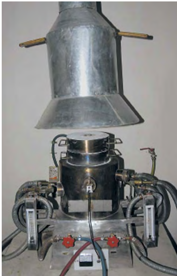
Figure 42. This is one of five furnaces used by Magic Stone Madagascar to heat treat corundum. Photo by Brendan Laurs.
