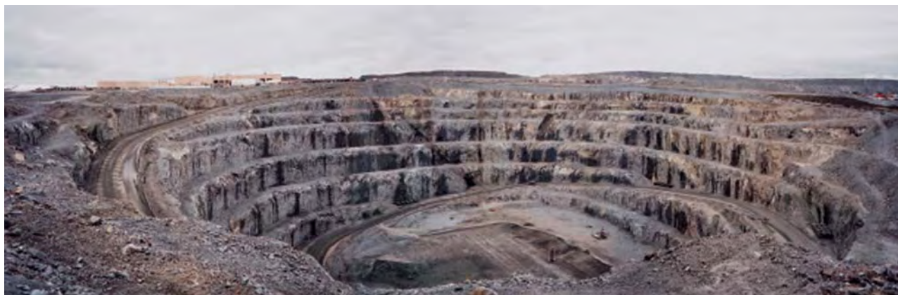
Figure 2. The Koala kimberlite at Ekati is visible as the dark-colored rock in the center of the open pit. Each bench is about 30 m high. Photo by Mary L. Johnson, June 2003.
