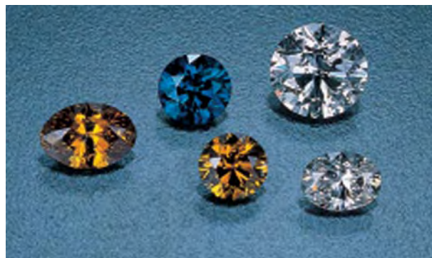
Figure 13. The synthetic diamonds shown here (0.29–0.78 ct) are among those GE produced experimentally in the 1970s. Photo by Robert Weldon, © GIA.
