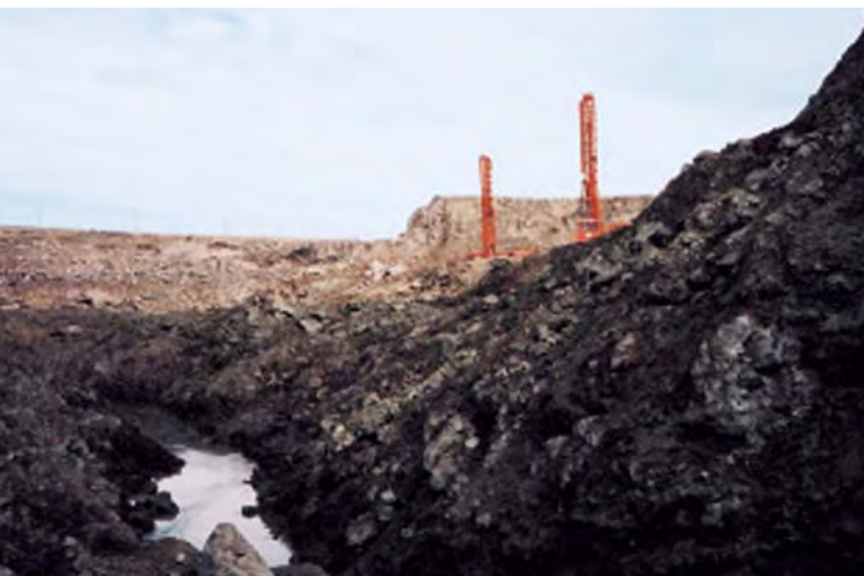
Figure 3. At Diavik's A154S pit, two orange cranes pump explosives into the 370-m-level bench. The dark rock in the foreground is diamondiferous kimberlite. Photo by Mary L. Johnson.
