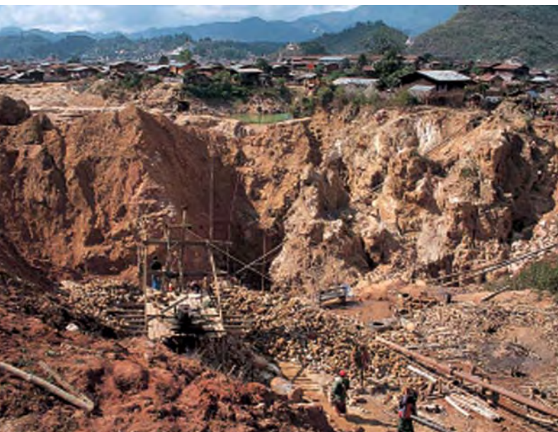
Figure 18. Rubies are recovered from this large pit at the Phau Htoke Khan mine, near Spider Hill in Mogok. The structure in the left center is a headframe used to raise material from the bottom of the pit. Photo by O. Galibert.
