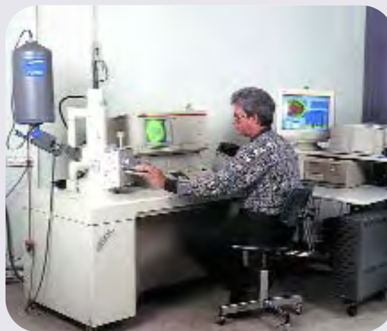
Figure A-1. The scanning electron microscope used for this study was equipped with an energy-dispersive X-ray spectrometer, for analysis of elements ranging from Be to U. Photo by M. K. Sukhanov.
