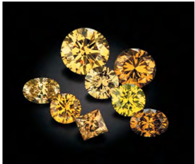
Figure 38. Iljin Diamond Co. is producing a range of colors through the HPHT treatment of type Ia diamonds (here, 0.4–2.0 ct). Photo © Robert Weldon/Professional Jeweler.
