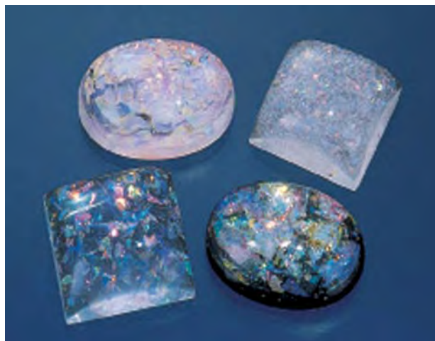
Figure 35. “Mermaid Crystal” is a new manufactured opal simulant that is available with either pinfire or broadflash “play-of-color.” The cabochons shown here range from 15.79 to 19.61 ct. Courtesy of Renato Rossi; photo by Maha Tannous.
