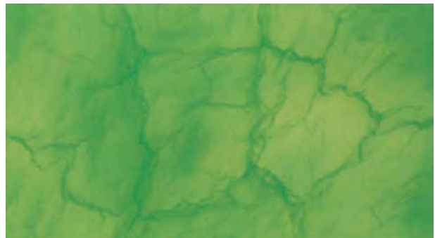
Figure 10. As Crowningshield reported more than 40 years ago, color concentrations in the surface-reaching cracks of jadeite jade are proof that the piece has been dyed. Photomicrograph by John I. Koivula; magnified 5×.
