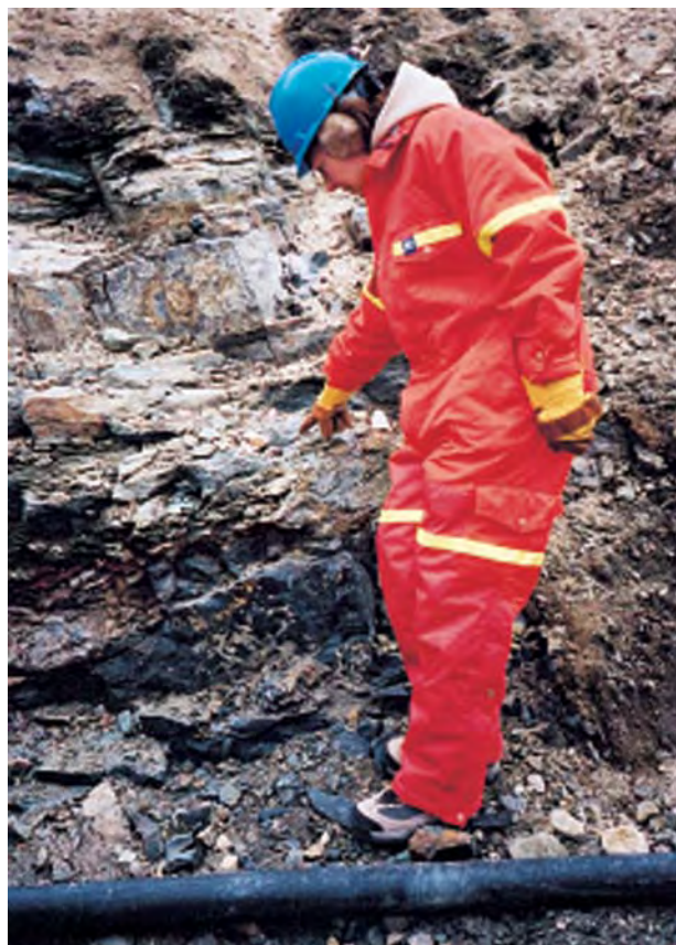
Figure 5. The diamondiferous kimberlite dike at Snap Lake averages only a few meters thick. Here, Dr. Melissa Kirkley, De Beers Canada Exploration, points out a xenolith in the dike; the upper contact of the dike with the host rock is at the level of her head. Photo by Mary L. Johnson.
