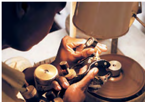
Figure 41. At the recently expanded facility owned by Magic Stone Madagascar, sapphires and rubies from that country are being cut using customized equipment. Photo by Brendan Laurs.
